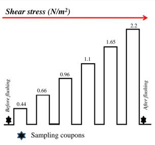
Fig. 3: Incremental shear stress applied to each loop after 28 days biofilm development.
