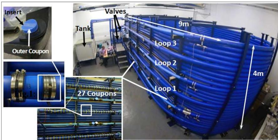
Fig. 2: Temperature controlled pipe-test facility at Sheffield University. Coupons are inserted along the length of each loop to allow for subsequent biofilm removal and examination.
