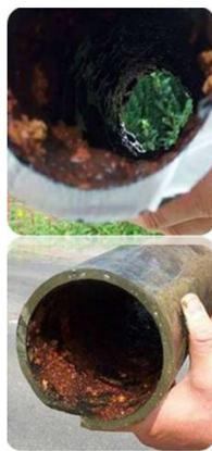
Fig. 1: Biofilm development within drinking water pipes.
