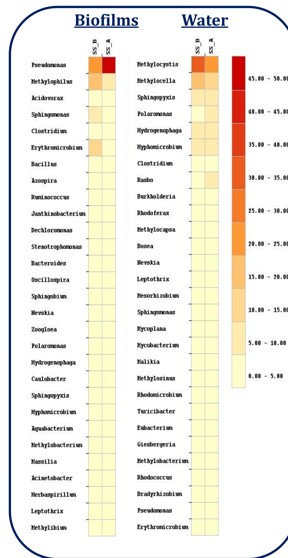
Fig. 6: Heatmaps showing the percentages of the most abundant species at genus level within bulk water and biofilms
