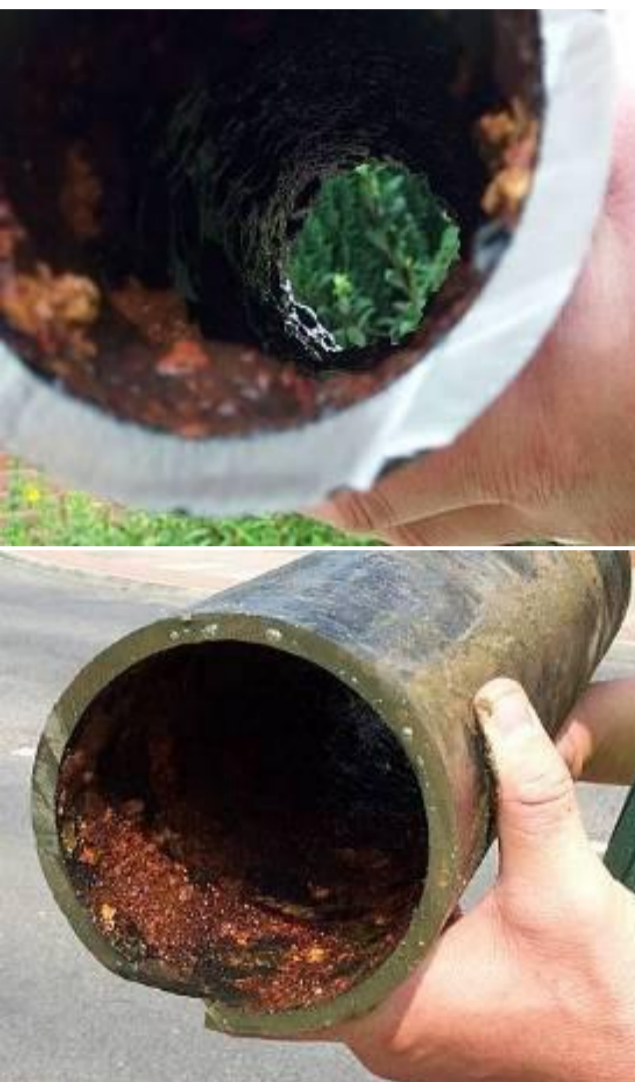
Fig. 1: Biofilm development within drinking water pipes
