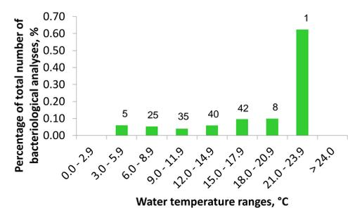
Fig. 4: Percentage of bacteriological failures with no known cause per total number of bacteriological analyses grouped by water temperature between 2008 and 2011. The number of failures per temperature range is presented above each bar.
