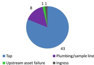
Fig. 2: Number of single causes identified by cause of failure.
