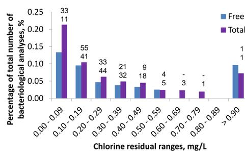
Fig. 3: Percentage of bacteriological failures with no known cause per total number of bacteriological analyses grouped by free and total chlorine residual between 2008 and 2011. The number of failures per chlorine residual range is presented above the bars, from top: Free, Total; - = no failures in this range.
