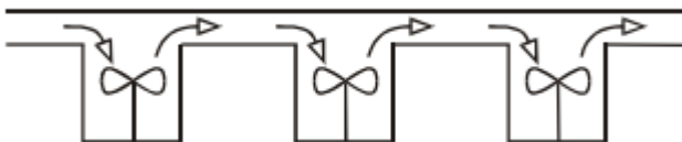
Figure A2. Representation of mixing zones in aggregated dead zone model (after Young and Wallis, 1986)
