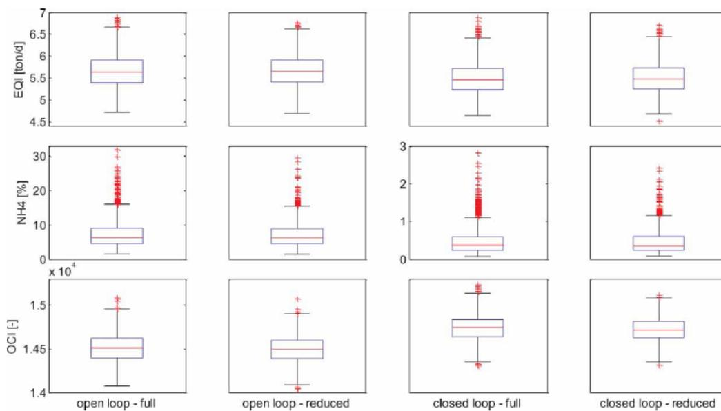
**Figure D1.** Whisker box-plots of the three evaluation criteria of BSM2 examining parametric uncertainty using a reduced number of parameters
