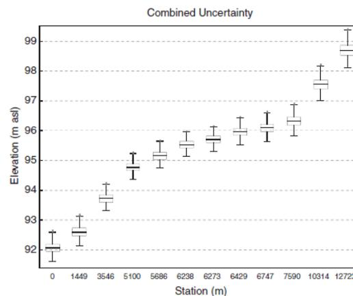
**Figure E4.** Range of water surface elevation (Box plots with minimum and maximum values, first, second and third quartiles), due to the combined effect of input data and model parameters uncertainty
