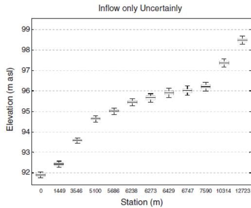
**Figure E2.** Range of water surface elevation (Box plots with minimum and maximum values, first, second and third quartiles), due to the input data uncertainty
