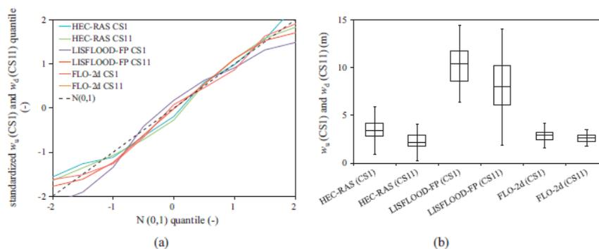
**Figure E1.** Simulated water depths ( $w_u$ , upstream and  $w_d$ , downstream cross-section) derived from several model structures: a) probability functions and b) box plot
