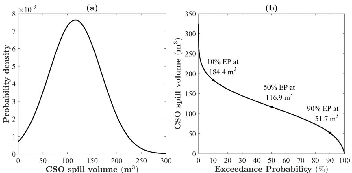
**Figure C1.** CSO volume probability density (left) and exceedance probability (right) derived by Monte Carlo analysis
