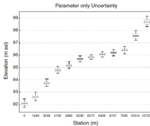
**Figure E3.** Range of water surface elevation (Box plots with minimum and maximum values, first, second and third quartiles), due to the model parameters uncertainty
