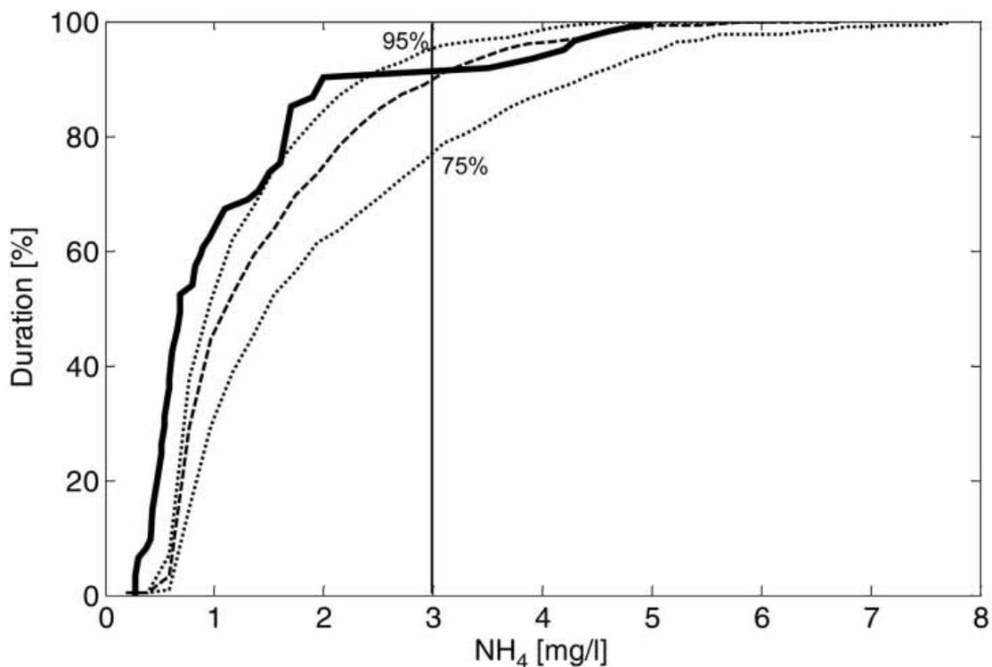
**Figure D2.** Observed cumulative curves of  $\text{NH}_4$  effluent (solid line) and simulated uncertainty band (5%, 50% and 95%) using Monte Carlo technique
