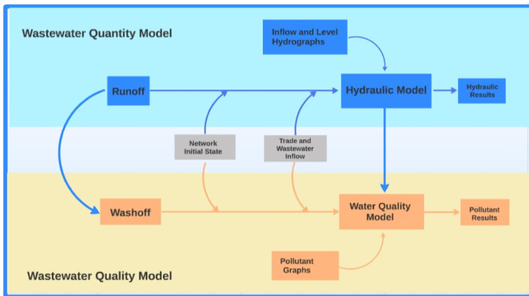
**Figure 3.** InfoWorks ICM<sup>®</sup> Model Structure (adapted from InfoWorks ICM<sup>®</sup> help)
