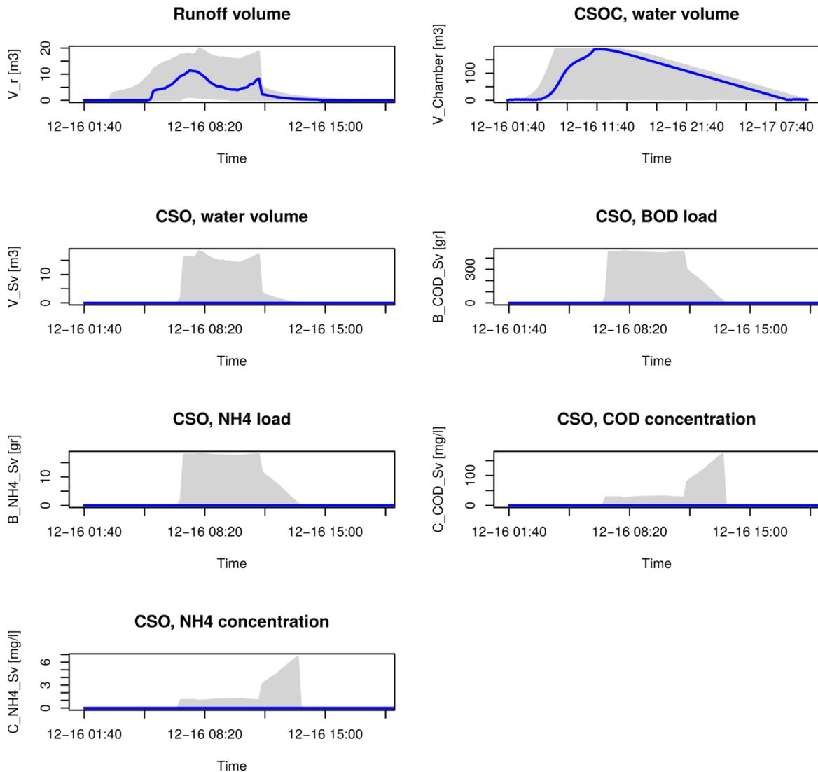
Figure 6. Output from model Level 1. Prediction value (blue line) and boundary of the 90 percent confidence interval (gray band). Goesdorf sub-catchment.
