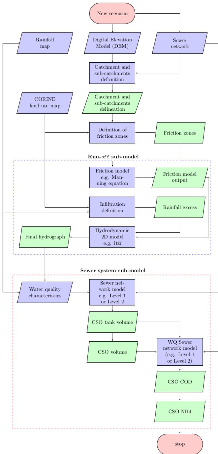
Figure 4. Work flow for the integrated rainfall-runoff and sewer system modelling.
