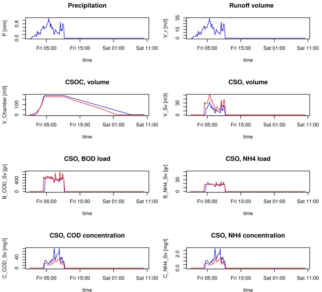
Figure 5. Comparison deterministic simulations for the integrated rainfall-runoff and sewer system models. EmiStatR (blue line) and CMM (red line). Goesdorf sub-catchment.
