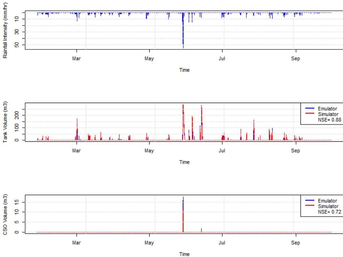
**Figure 2.** Validation of emulator vs. detailed simulator for simulation of total tank volume and CSO volume for one-year duration.
