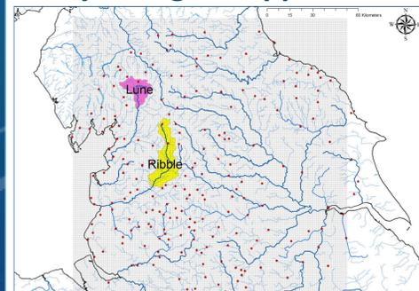
Figure 9 - The two selected catchments are represented with the radar grid and the rain gauges (as red dots), together with the river network.
