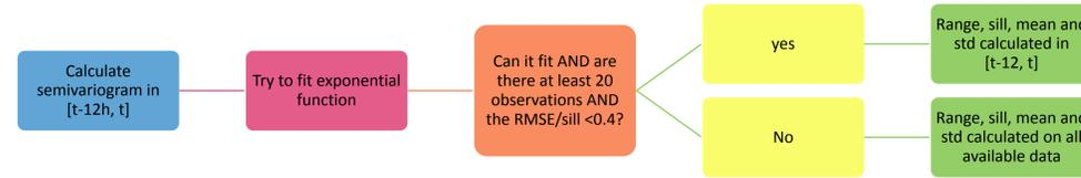
Figure 5 - The scheme represents the method followed to calculate error characteristics in real time, when possible. Usually when it is not possible it is because there is too little rain, therefore using the average statistics does not have a big impact.
