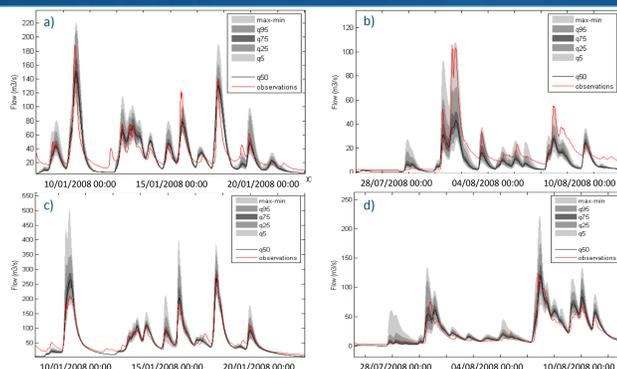
Figure 10 - The output of the PDM model for the Lune (a,b) and Ribble (c,d) basin, using the ensemble error compared with flow observations for a winter event (6 January 2008 - 27 January 2008) (a,c) and for a summer event (24 July 2008 - 14 August 2008) (b,d).
