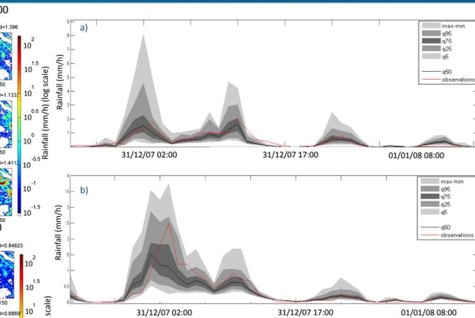
Figure 7 - Example of ensemble members compared with the original radar (in the red square) before (a) and after (b) correction. The event refer to the 1st January 2008 at 05:00.
