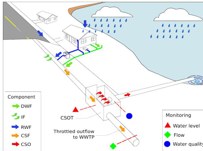
Figure 1. Main components of the EmiStat model: 1) Dry Weather Flow (DWF) including Infiltration Flow (IF); 2) Pollution of DWF; 3) Rain Weather Flow (RWF); 4) Pollution of RWF; 5) Combined Sewage Flow (CSF) and pollution; and 6) Combined Sewer Overflow (CSO) and pollution. (Background adapted from: Sanitary-District, 2015).
