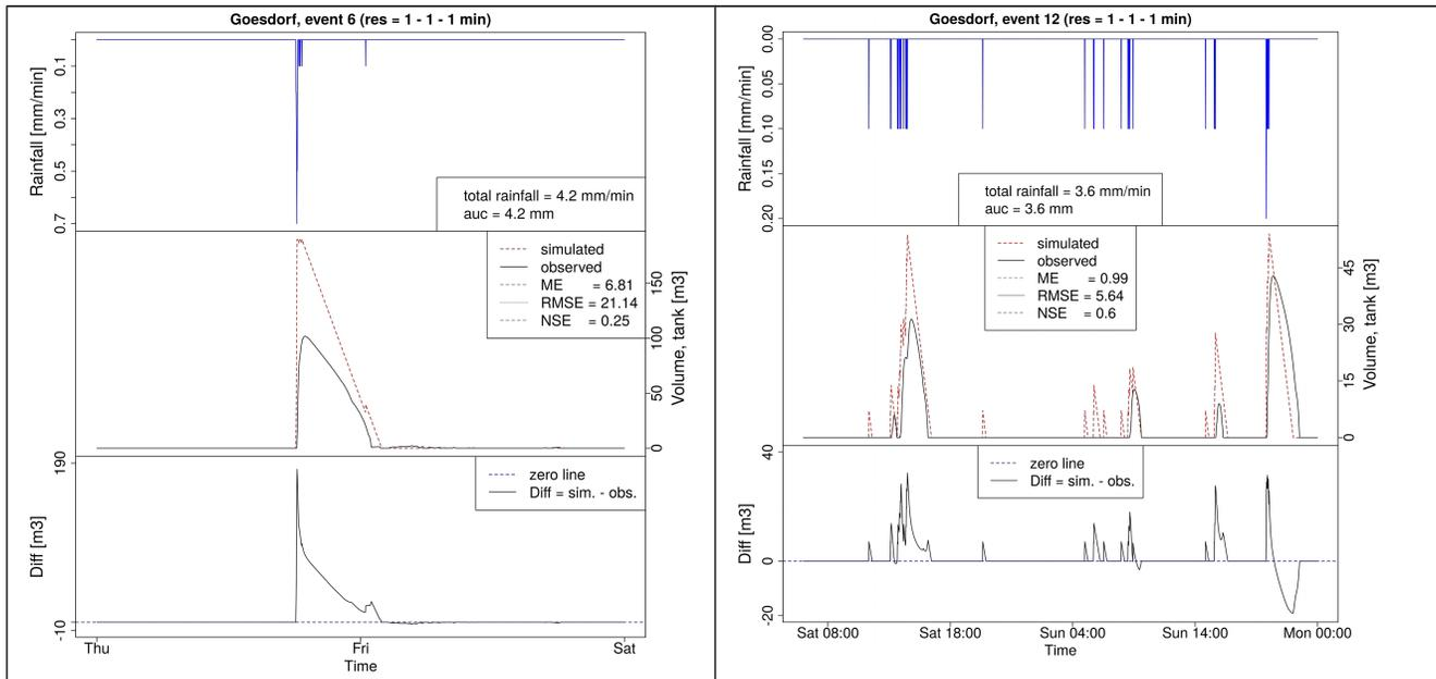
**Figure 4.** Accuracy assessment of the EmiStat-R model simulating volume in the CSOT for rain events without CSO at Goesdorf station; (a) event 6, rain from 19/05/2011 00:00:00 to 21/05/2011 00:00:00; (b) event 12, rain from 31/05/2011 00:00:00 to 01/06/2011 12:00:00.
