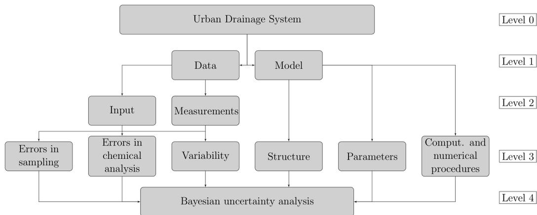
**Figure 2.** Proposed framework for uncertainty analysis in urban drainage modelling.
