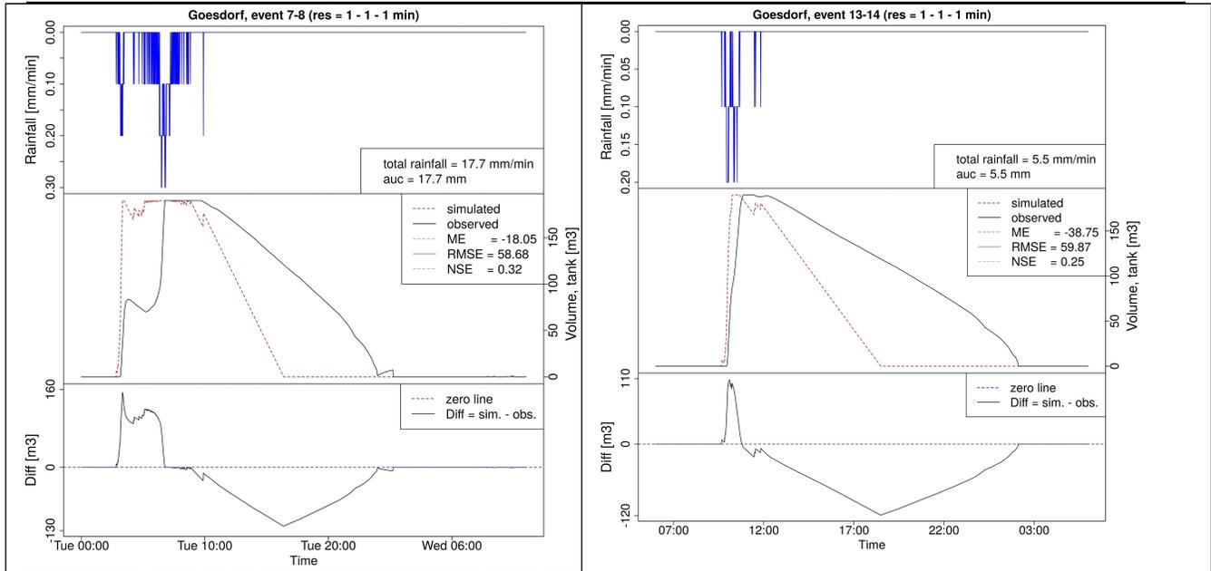
**Figure 5.** Accuracy assessment of the EmiStat-R model simulating volume in the CSOT for rain events with CSO at Goesdorf station: (a) event 7-8, rain from 18/06/2011 06:00:00 to 20/06/2011 00:00:00; (b) event 13-14, rain from 22/06/2011 06:00:00 to 23/06/2011 06:00:00.
