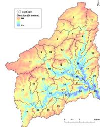
Figure 2: Subbasins and 30 meter resolution DEM
