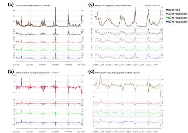
Figure 4: Mean (a) daily and (c) monthly discharge. Difference between simulated and observed (b) daily and (d) monthly discharge data.
