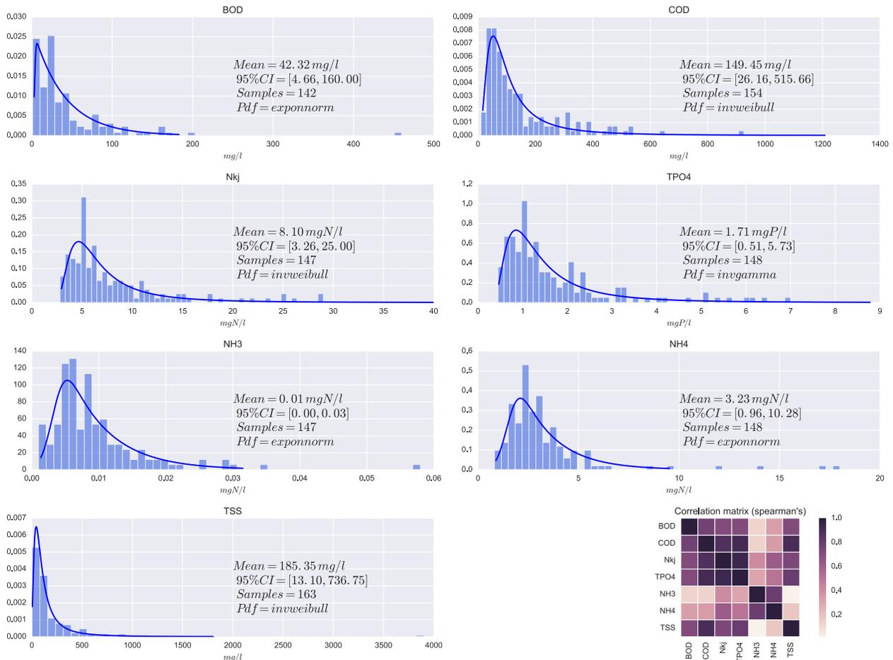
Fig 1 Histograms and correlation matrix of measured data, mean and 95% confidence intervals. Blue solid line; fitted pdf.
