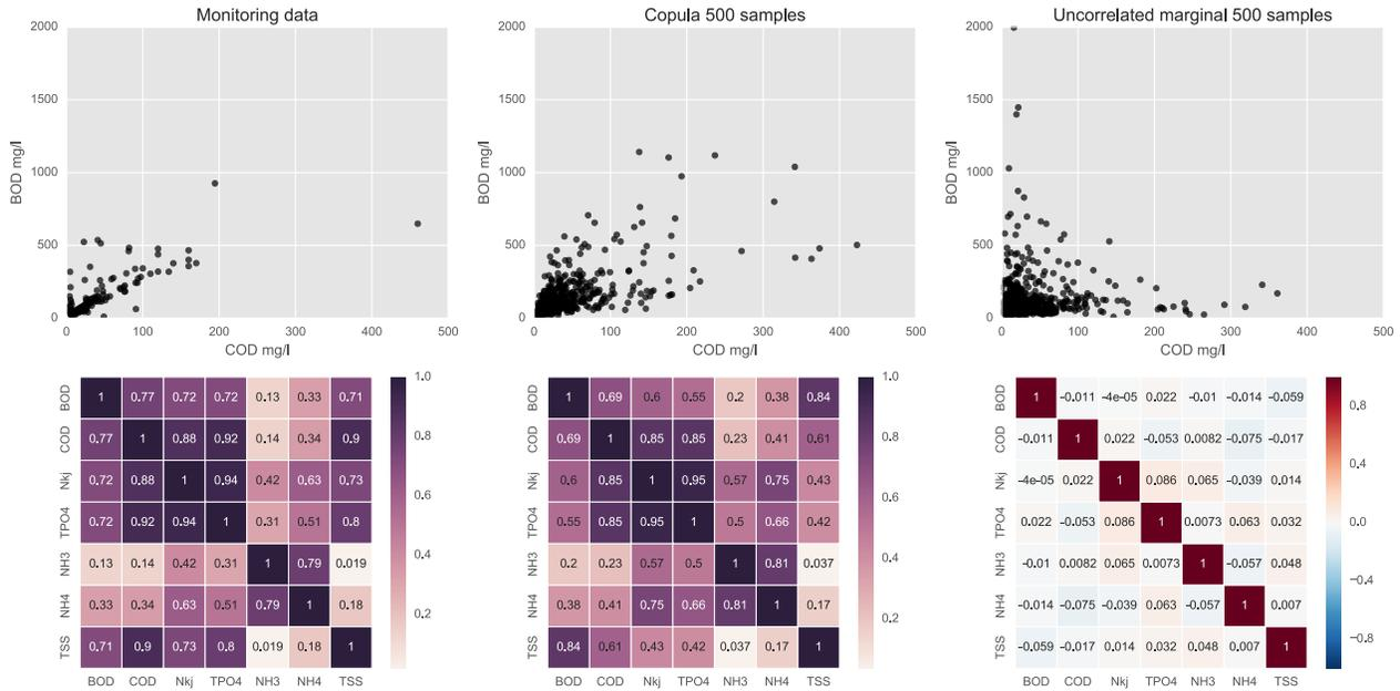
Fig 2 Comparison of measured data, GC and random sampling from marginals. Above, scatter plot for BOD-COD. Below, correlation matrix.
