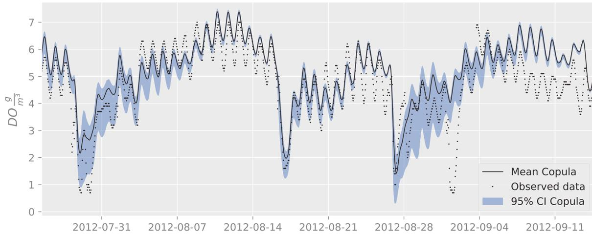
Fig 3 DO at the river (~17 km downstream of the WWTP). Observations vs simulated (GC).
