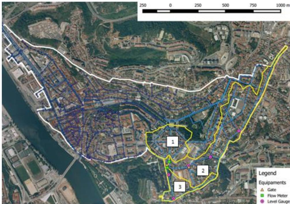
Figure 2 Zona Central catchment with the new location of level and flow sensors and possible gate locations.
