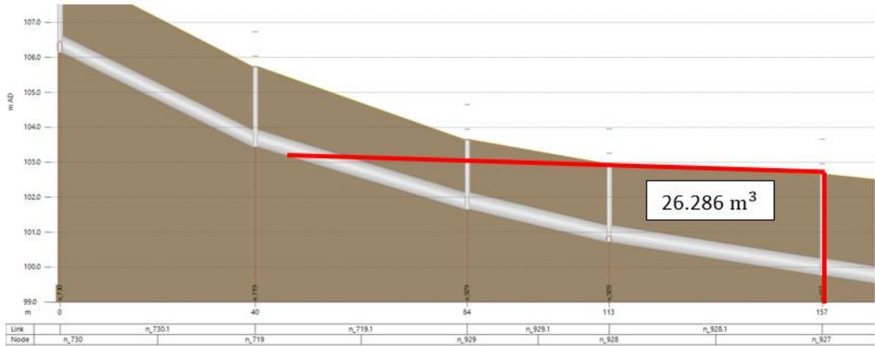
Figure 16 Longitudinal profile perspective showing the pipes available for storage volume (Infantaria)
