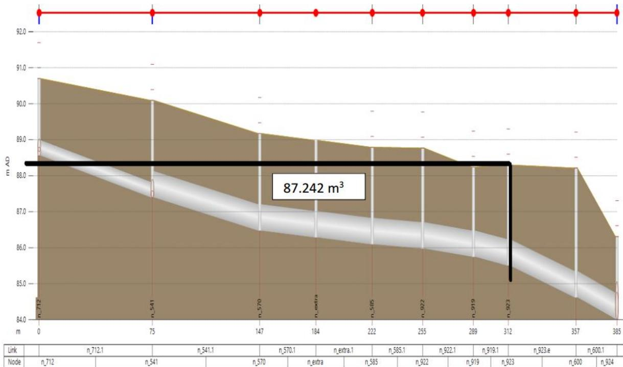
Figure 15 Longitudinal profile perspective showing the pipes available for storage volume (Julio Henriques)
