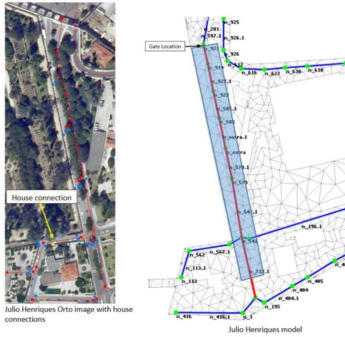
Figure 7 Av. Júlio Henriques: Orto image with house connections and Julio Henriques network from the hydraulic model in InfoWorks
