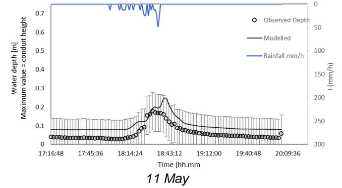
Figure 3 Example of Calibration and validation of data in Av Julio Henriques flowmeter.
