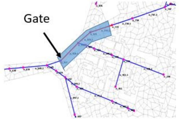
Figure 11 Rua da Infancia 23 Orto image with house connections and network from the hydraulic model in InfoWorks
