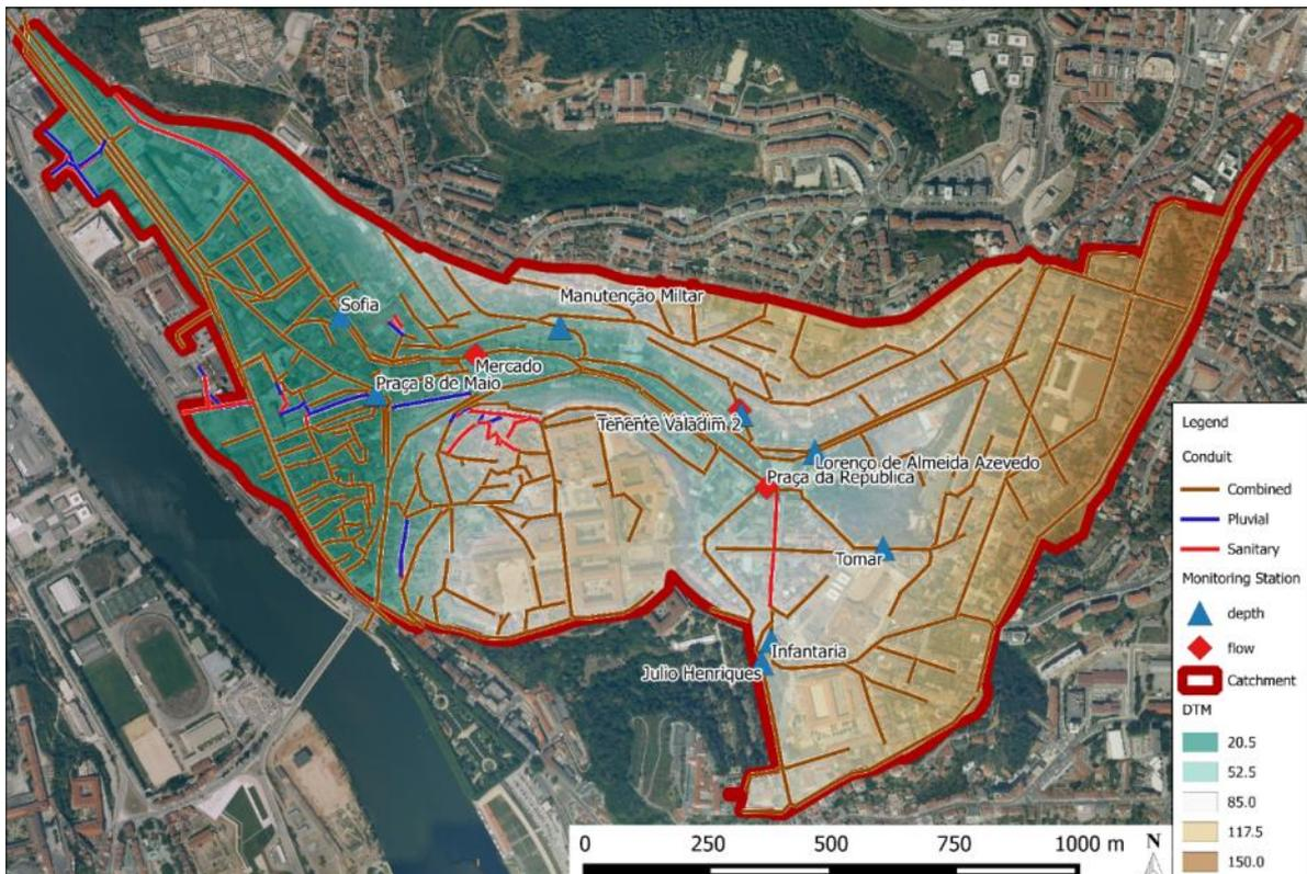
Figure 1 Zona Central catchment with location of level and flow sensors
