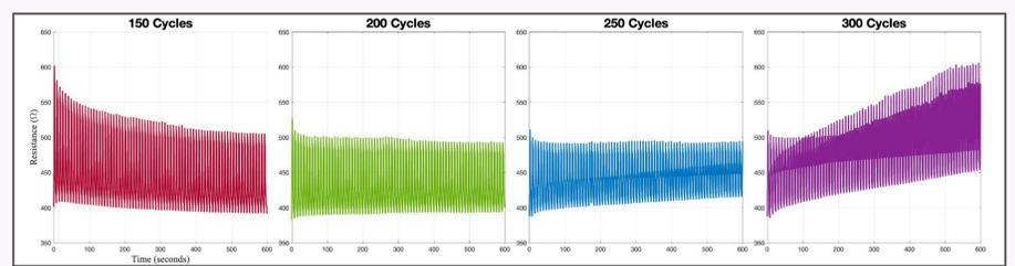
Fig 5. Initial response of sensor different number of cycles (Using Resistance - Time graph)
