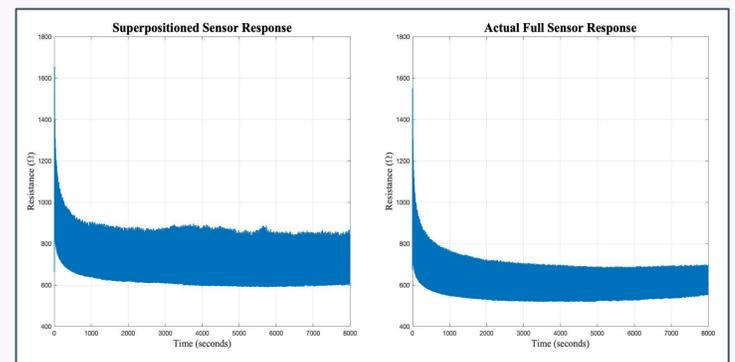
Fig 6. Result of superpositioning of silver and graphite sensor responses (left) and comparing with a full silver-graphite sensor response (right)
