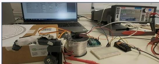
Fig 3. Experimental setup to measure strain during continuous bending and stretching motion of a finger
