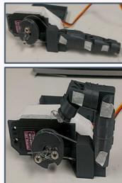
Fig 2. A single finger model to stimulate bending motion
