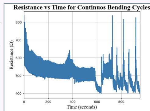
Fig 7. A snapshot of response of strain sensor to bending and relaxation movement of a single finger
