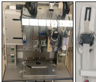
Fig 1. 3-D pressure based printer for printing sensor on glove (left). A sample 3-D printed graphite-silver based strain sensor
