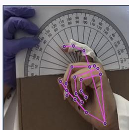
Fig 4. Experimental setup to identify angle of bending to correlate resistance value for training ML model
