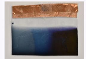
Fig.5 Differential appearance of conductive hydrogels from oxidised and reduced electrodes after bipolar experiment (Light and Dark)
