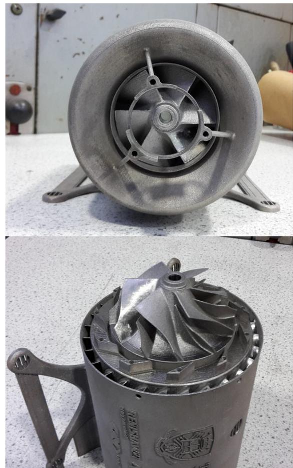
Fig. 2. Photograph of the 3DP jet engine produced by undergraduate students.
