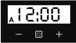
Press mode button
