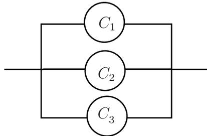
Find the reliability of the system where  $R_1 = 0.2$ ,  $R_2 = 0.3$  and  $R_3 = 0.4$ .
