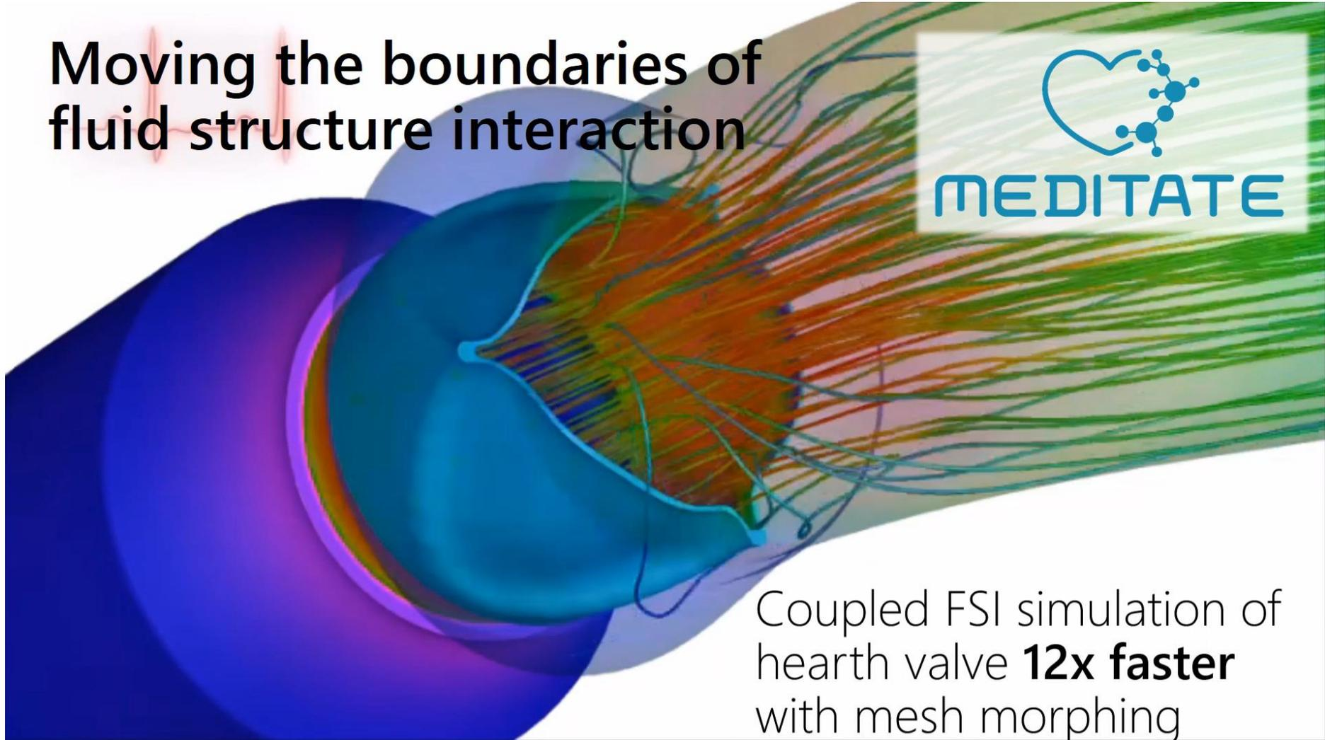
Coupled FSI simulation of heart valve **12x faster** with mesh morphing
