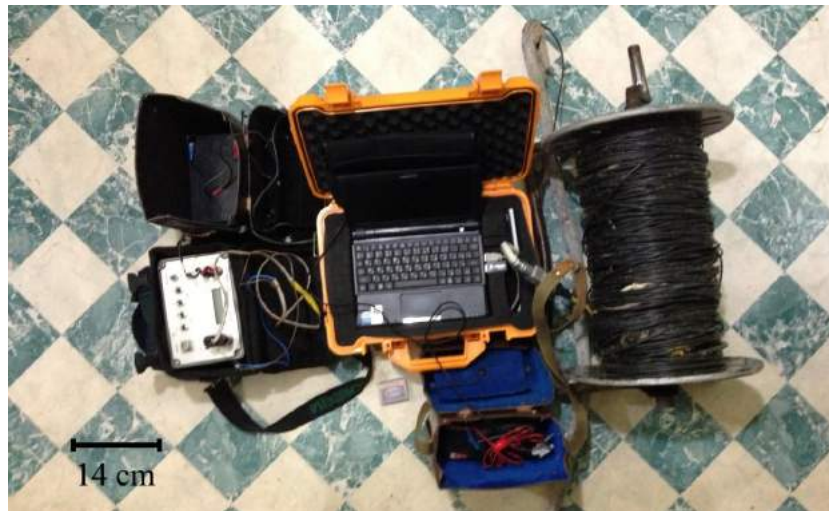
Fig.1. MISC field equipment for investigations by DC resistivity and IP methods (GI KSC RAS)
