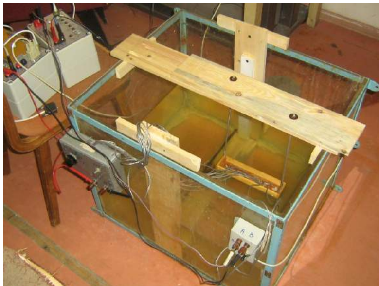
Fig.2. Installation for physical modeling and testing of DC resistivity and IP multi-electrode survey systems
