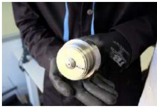
Figure 2. Through bulkhead initiator, showing the 4-nozzle configuration.
