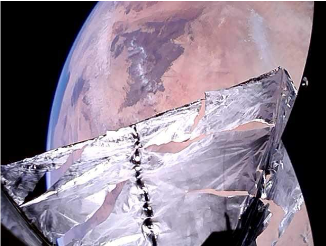
Fig. 2. PW-Sat2 onboard camera photo with torn structure of deorbit sail.
