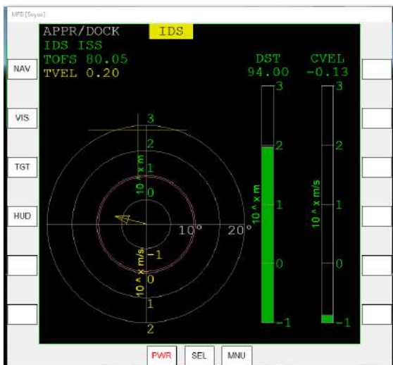
Figure 3: The "Docking" MFD helps keep track of the docking target and align for approach.
