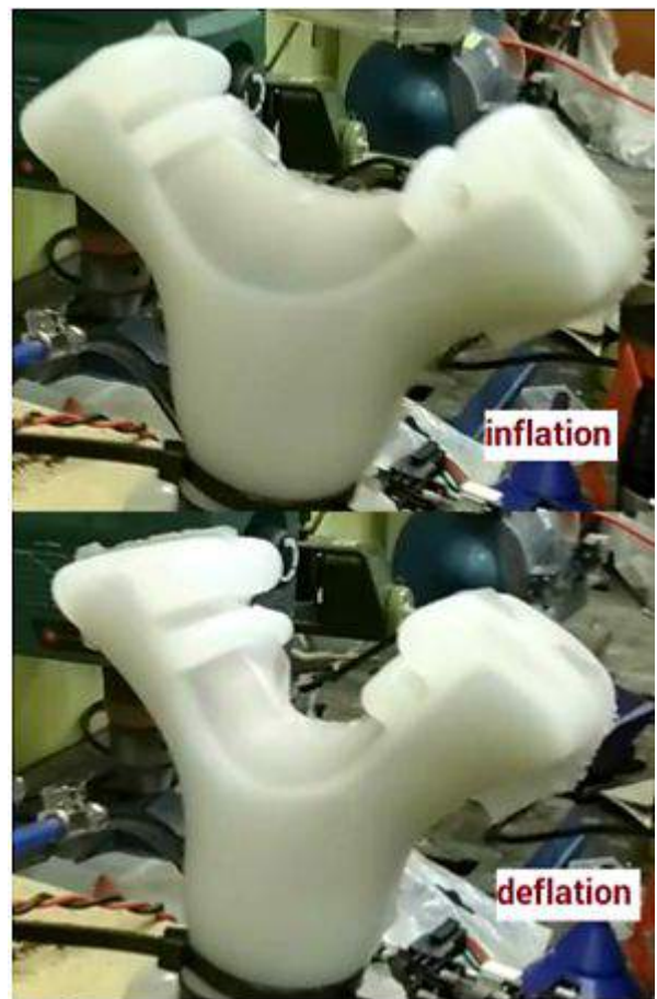
Fig. 4. End effector in two states (prototype)
