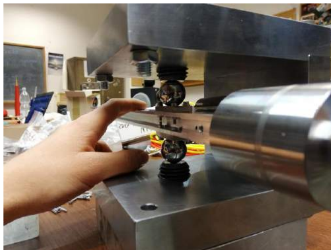
Fig. 4. Torosional pendulum based thrust stand developed for propulsion system test campaign, during its itegration.
