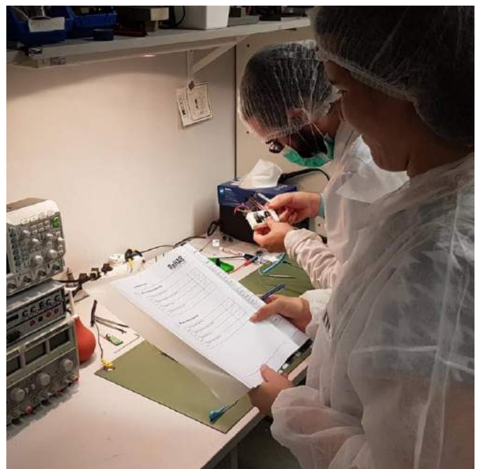
Fig. 5. Working on flying hardware in 'grey' lab area to prevent contamination and ensure high quality
