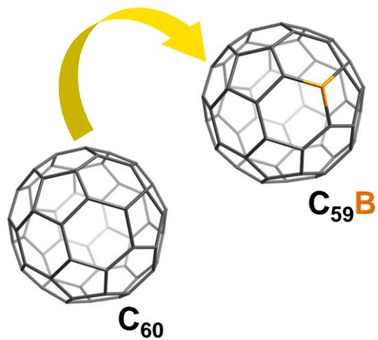
*The heterofullerenes,  $C_{59}B$ , is directly synthesized from pristine  $C_{60}$  by atom exchange reactions with B.*
