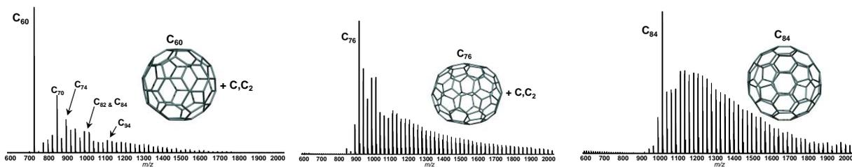
Comparison of growth patterns after exposure of  $C_{60}$ ,  $C_{76}$ , and  $C_{78}$  to carbon vapor, under optimal growth conditions. The same growth trends are observed indicating single mechanistic route. Importantly, absolutely no  $C_{60}$  forms via the growth processes of larger fullerenes. Thus,  $C_{60}$  forms by CNG from smaller fullerenes and is shown to be most resistant to carbon incorporation, further solving why  $C_{60}$  forms as the most abundant fullerene.
