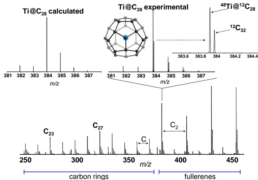
*The tiny  $T_d$ - $C_{28}$  fullerene is grown a titanium atom.*
