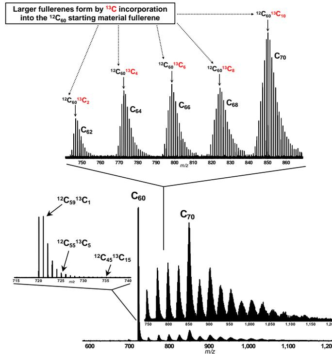
Exposure of  $C_{60}$  to pure  $^{13}\text{C}$  vapor tracks growth;  $C_{60}$  is clearly shown to grow bottom-up into larger fullerenes by incorporation of  $C_2$  and  $C$ .
