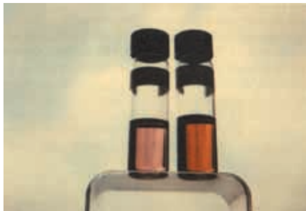
Fig. 26. Chromatographic separation of the red extract by Taylor resulted in a magenta C_{60} fraction (left) and a red C_{70} fraction (right).
