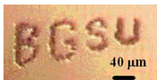
Figure 7. Optical microscope image of a microstructure obtained through the TPA-photoinitiated polymerization of TMPTA with 1%wt. of 1 .
