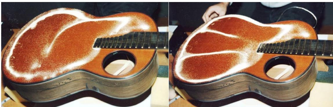
Sand vibrational patterns on Kasha classical guitars at two frequencies (a, b), showing extended use of soundboard by long bass-coupling bars permitted by off-center soundhole.
