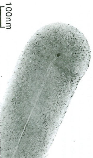
Fig. 2. Vapour-grown carbon fiber showing relatively early stage of growth; at the tip the seeded Fe catalytic particle is encapsulated.
