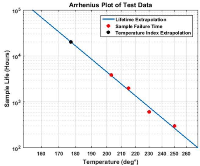
Fig. 4: Lifetime as function of temperature for 4 samples at constant temperature
