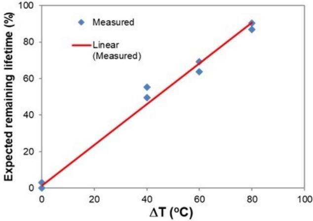
Fig. 7 Expected remaining lifetime at the time of failure as function of  $\Delta T$
