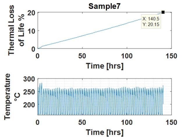
Fig. 5 Thermal cycling experimental results for Samples 2 to 7: samples' temperatures and thermal loss of life
