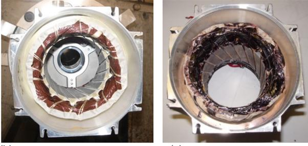
Fig. 2 Machine sample (a), prior to ageing (b) and after failure (c)
