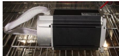
Fig.9 Stator sample inside the temperature controlled chamber
