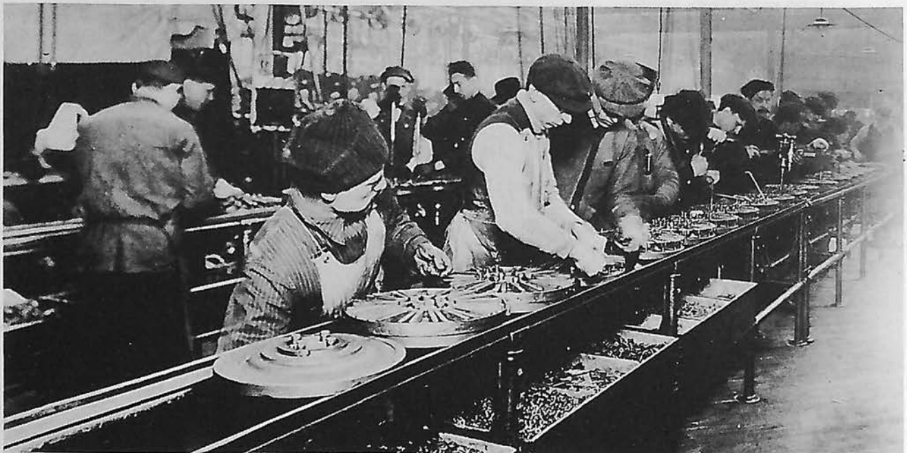
Old methods of production give way to the new. Above: the Smith's shop, Britannia Railway Carriage Works, Saltley. Below: the first assembly line, Ford's Park Plant, 1913.
