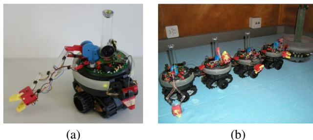
Fig. 1. The swarm-bot concept: (a) a mobile module called *s-bot*, fully autonomous in perception, control, action, and power, capable of approaching and assembling with its teammates, (b) a modular robot called *swarm-bot*, composed of four *s-bots*, manipulating an object.
