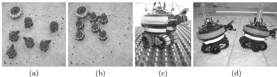
**Fig. 2.** Initial (a) and final (b) configuration of six s-bots self-assembling with the prey on flat terrain. Types of rough terrain: the *moderately rough terrain* (c), and the *very rough terrain* (d).
