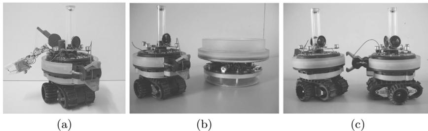
**Fig. 1.** (a) A single robot. Self-assembly with (a) an object, and (c) a teammate.
