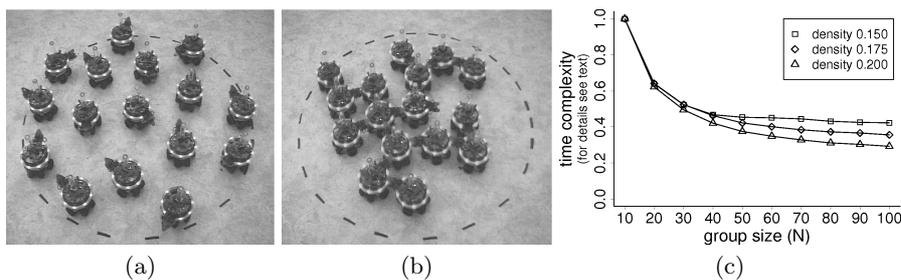
**Fig. 3.** Self-assembly in a robotic swarm. Initial (a) and final (b) configuration of 16 physical s-bots put in a circle of radius 50 cm. Time complexity (c) for groups of 10 to 100 s-bots put in a circle around the prey (for different initial robot densities): average time (over 200 trials in simulation) it took an s-bot to connect, divided by the group size and scaled so that the performance for group size 10 equals 1.
