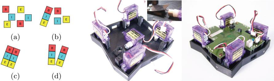
**Fig. 1.** Left: (a–d): illustration of the growth and replication process. Center/right: generic hardware prototype capable of simulating all aspects of the *e*-, *i*-, and *b*-modules. Center: squared base with four connection sides. The inset shows a hatch in the bottom plate, which controls the mobility of the module, which floats on an air table. Right: fully assembled prototype (battery removed).
