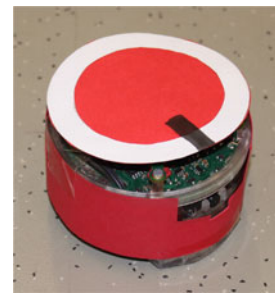
Fig. 8. Close view of the robotic platform used in the experiments. The e-puck is coated in red to be identifiable by other e-pucks. The marker on its top is used by the tracking system for the post-analysis.
