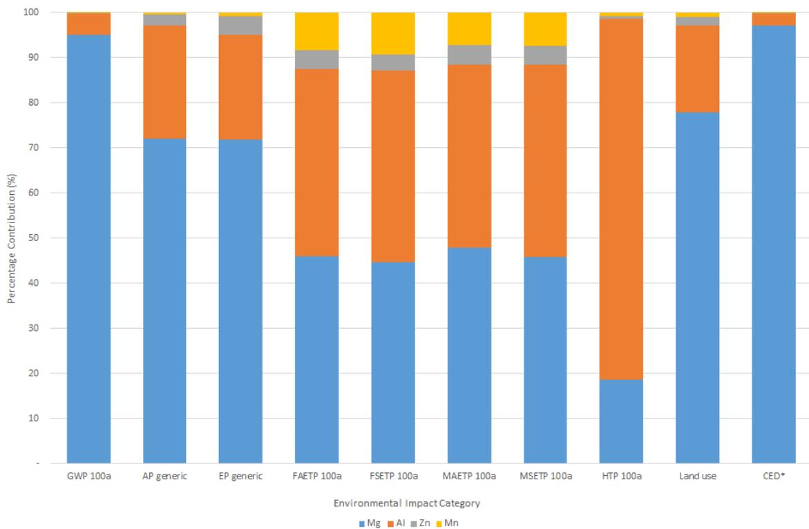
Figure 5 Percentage contribution of each alloying material of the AZ31 alloy for the environmental impacts investigated. \*Cumulative energy demand.
