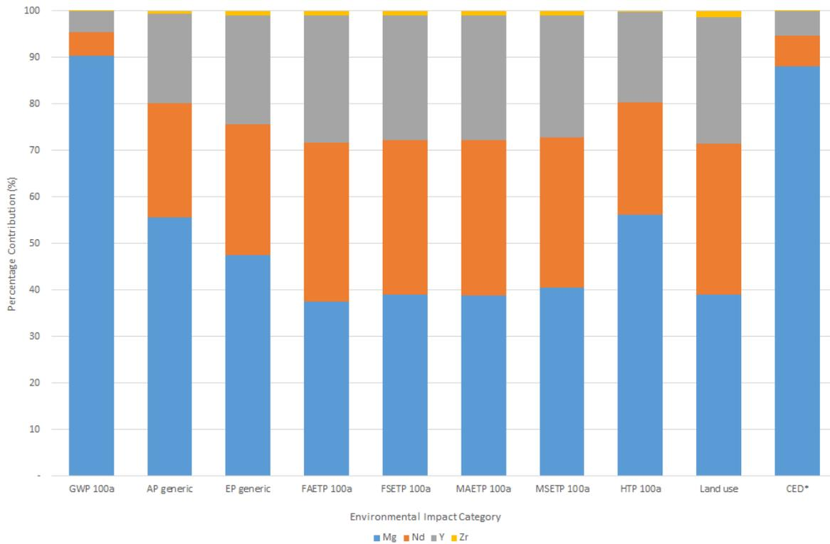
Figure 3 Percentage contribution of each alloying material of the WE43 alloy for the environmental impacts investigated. \*Cumulative energy demand.
