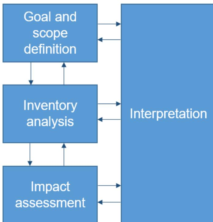
Figure 1 LCA framework [4]
