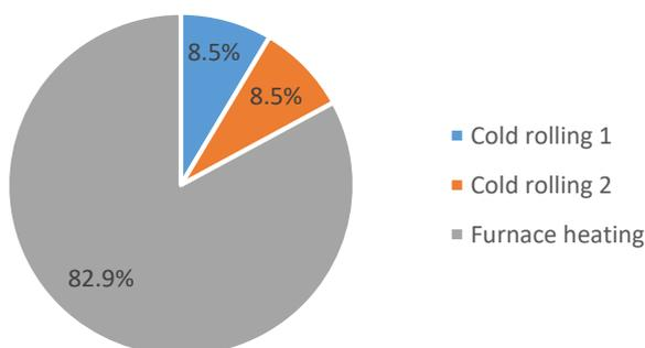
Figure 8 The percentage electrical energy contributions of each laboratory production process for all magnesium alloy compositions. The die casting process, performed prior to laboratory processing, is not included in this chart.
