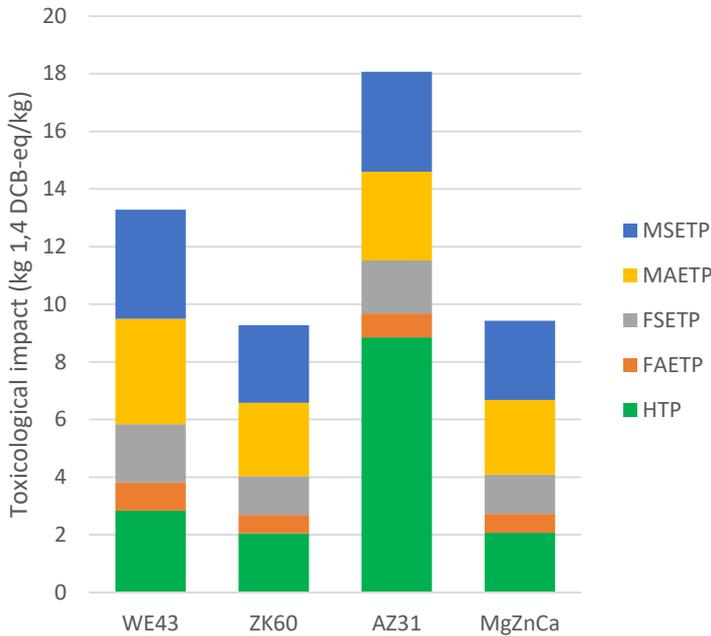
Figure 10 The total toxicological impact comparison for the WE43, ZK60, AZ31 and MgZnCa alloys.
