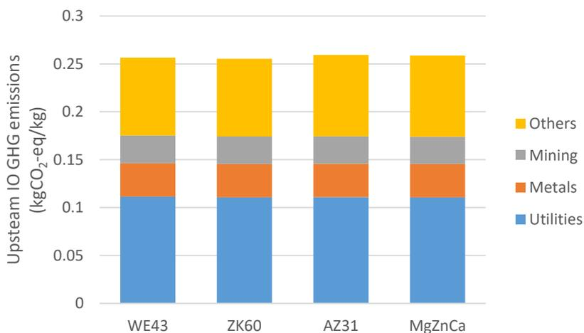
Figure 11 The upstream IO GHG emissions comparison for the WE43, ZK60, AZ31 and MgZnCa alloys.
