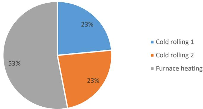
Figure 9 The percentage thermal energy contributions of each laboratory production process for all magnesium alloy compositions. The die casting process, performed prior to laboratory processing, is not included in this chart.
