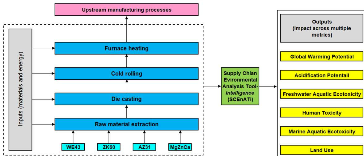
Figure 2 The system boundary of the magnesium alloy LCA; all process steps enclosed within the dotted lines are included in the LCA.
