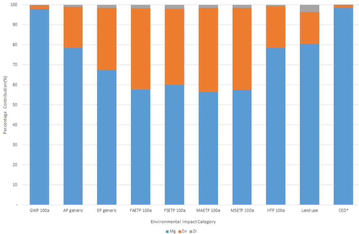
Figure 4 Percentage contribution of each alloying material of the ZK60 alloy for the environmental impacts investigated. \*Cumulative energy demand.
