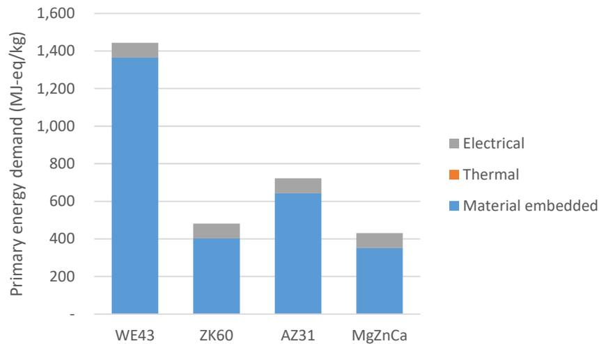
Figure 7 The primary energy demand comparison for the WE43, ZK60, AZ31 and MgZnCa alloys.
