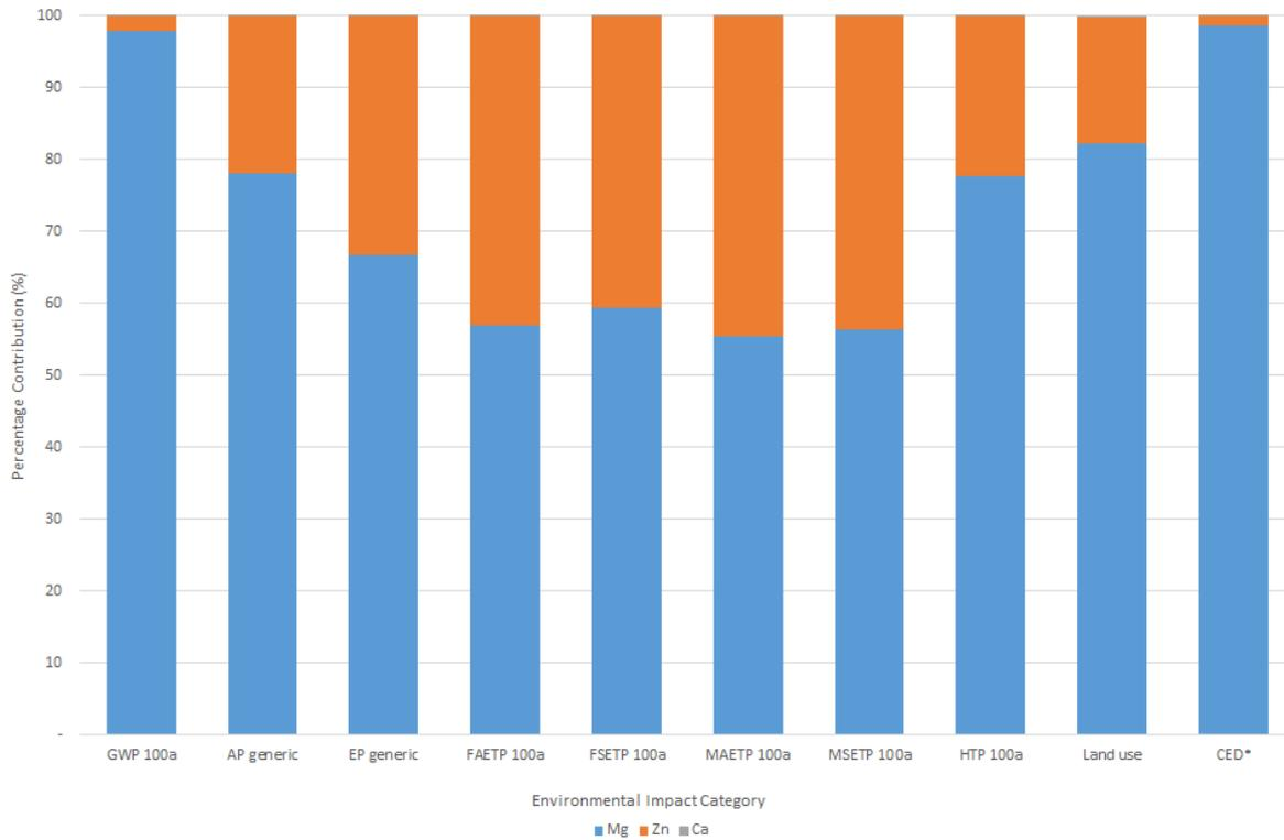
Figure 6 Percentage contribution of each alloying material of the MgZnCa alloy for the environmental impacts investigated. \*Cumulative energy demand.
