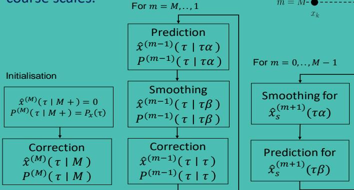
The algorithm can be broadly divided into three stages: initialisation, fine-to-coarse estimation sweep, and coarse to fine estimation sweep. Each step of the algorithm utilises the dynamical model of the system in forward time in square root implementation of the classical estimation procedures: Kalman filter prediction, measurement update, and RTS
