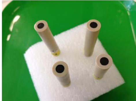
*Solid-contact electrodes after carbon nanotubes deposition and before membrane deposition.*
