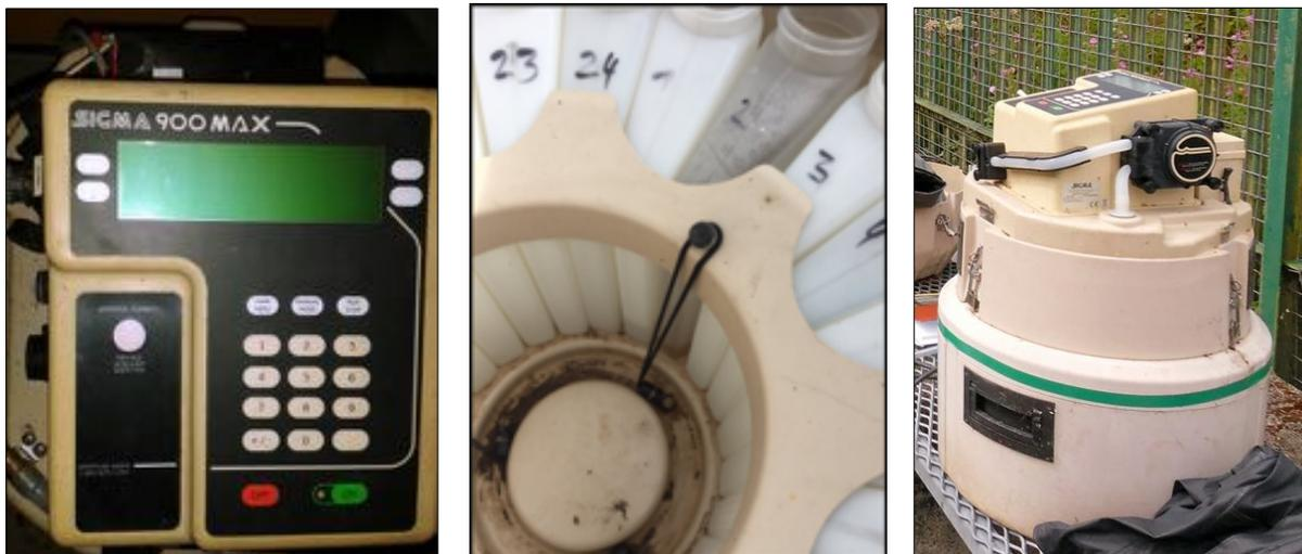
Figure 8. Automatic water sampler
