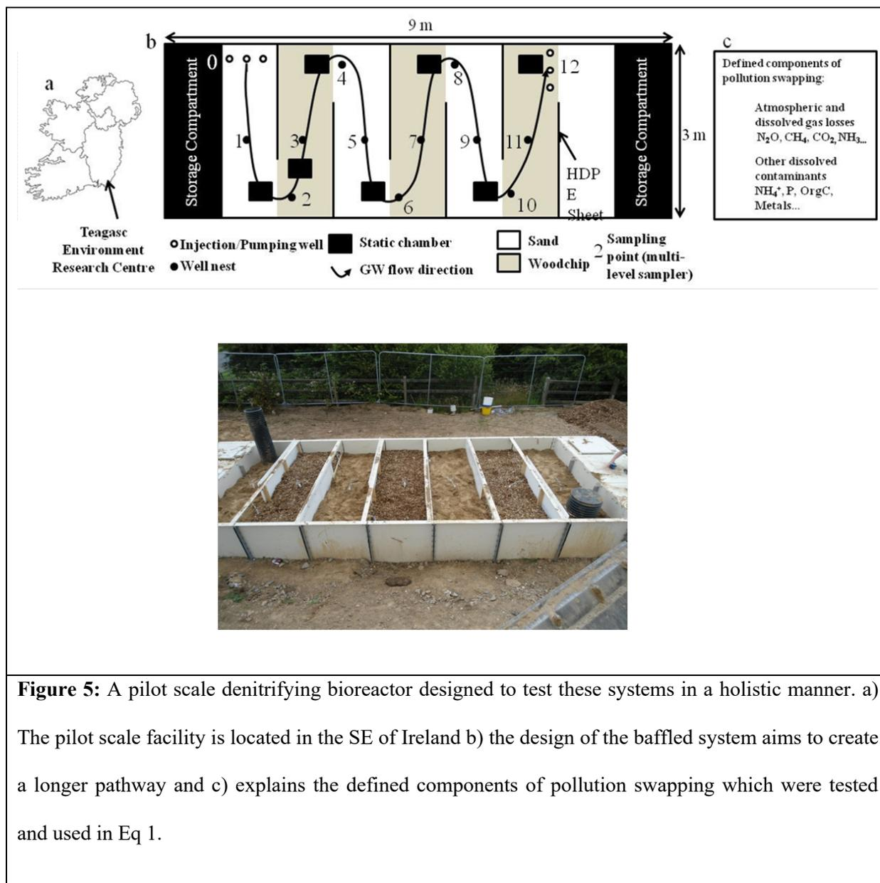
**Figure 5:** A pilot scale denitrifying bioreactor designed to test these systems in a holistic manner. a) The pilot scale facility is located in the SE of Ireland b) the design of the baffled system aims to create a longer pathway and c) explains the defined components of pollution swapping which were tested and used in Eq 1.
