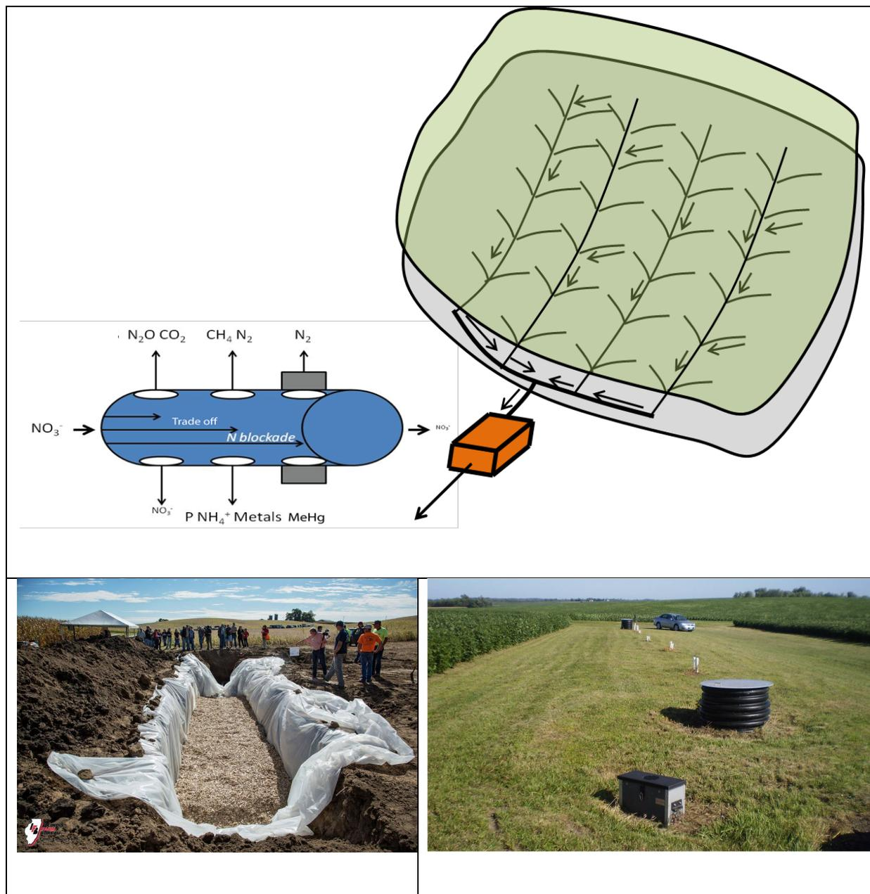
**Figure 1:** Top – concept of the location of a denitrifying bioreactor at the end of a tile drainage system. N blockade – this is a schematic of a leaky pipe which outlines the pollution swapping potential of systems even where N output is less than N input. Bottom – photo of a woodchip filter installation and a soil capped system.
