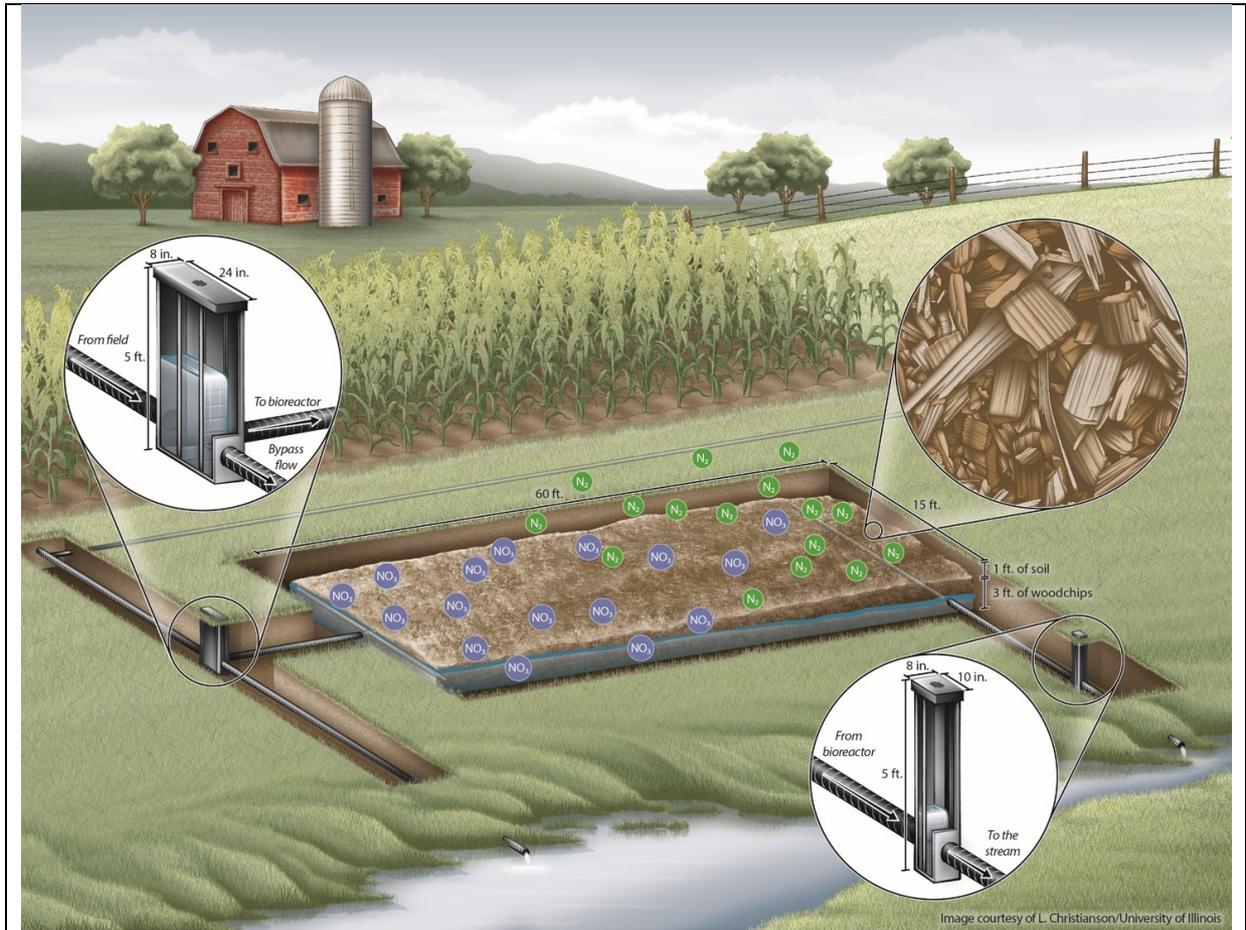
**Figure 8:** Generalized schematic of a denitrifying bioreactor to treat nitrate in subsurface drainage in the US Midwest. Credit: L. Christianson/University of Illinois.
