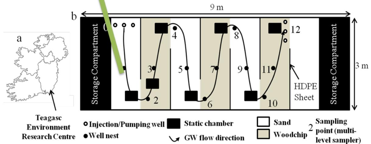
**Figure 6a:** Each of the cells has a series of multi-level piezometers to examine nutrient breakthrough at multiple depths. In addition, gas chambers were placed on top of the woodchip media over time to assess gaseous emissions. Such data is fitted into Eq 1.
