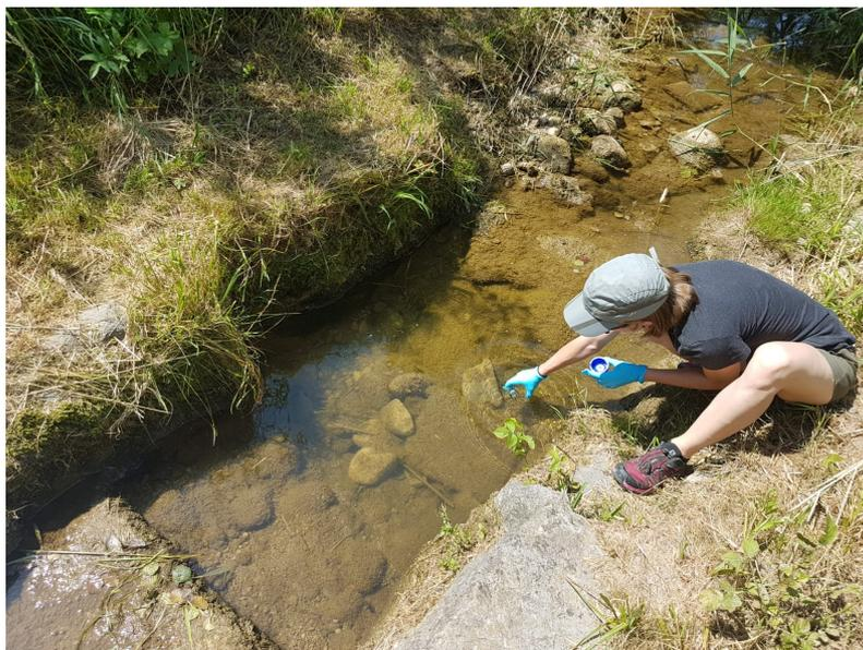
*Figure 3: Sampling for organic micropollutants in surface water: always use glass bottles and wear gloves!*
