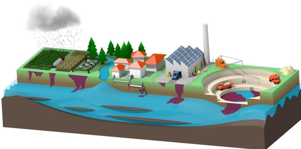
*Figure 1: Example conceptual model of a river catchment, including the presence of groundwater bodies and various anthropogenic influences*
