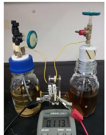
**Figure 2** Laboratory microbial fuel cell producing electricity from contaminated groundwater.
