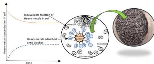
Figure 1 – Schematic of biochar effect on bioavailable fraction of heavy metals in soil.
