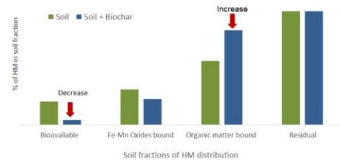
Figure 4. Generic distribution of metals in the different fractions of soils and the expected redistribution after biochar addition, based on the findings of (Lu et al. 2017).
