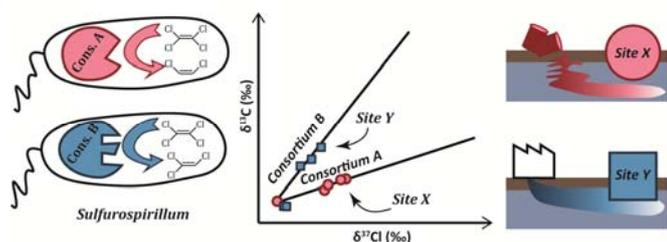
**Figure 3. Schematic summary of the results - Each "Sulfurospirillum-containing consortium" yields a distinct dual C-Cl isotope slope associated with PCE reductive dechlorination. Similar dual isotope slopes are observed for PCE reductive dechlorination in two different sites. Modified from Badin *et al.*, 2014**
