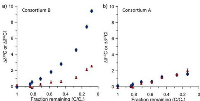
**Figure 2. Evolution of C and Cl isotope ratios with decreasing PCE remaining fraction for consortia A and B. Modified from Badin *et al.* (2014). Red triangles represent Cl isotopic ratios while blue circles represent C isotopic ratios.**
