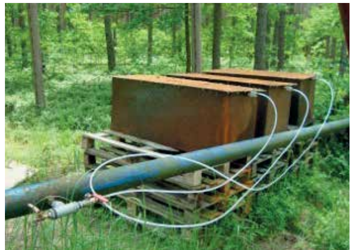
Fig. 4: Field demonstration of the PRB with the selected reactive materials
