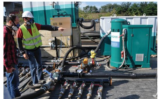
Figure 2. MPE vacuum extracGon pump.
