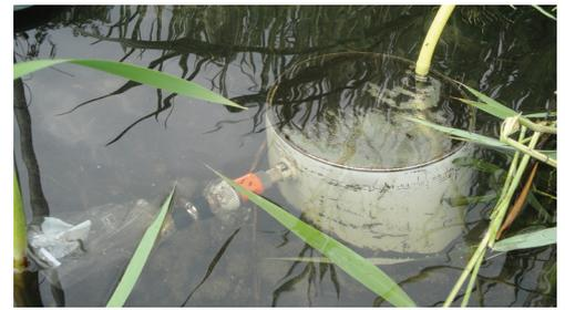
Figure 1. A typical seepage meter
