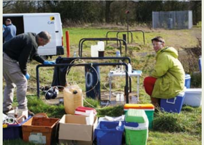
Figure 3. Collection of groundwater samples for hydrochemical and microbiological analysis of contaminant plume fringe, using a high-resolution multilevel groundwater sampler
