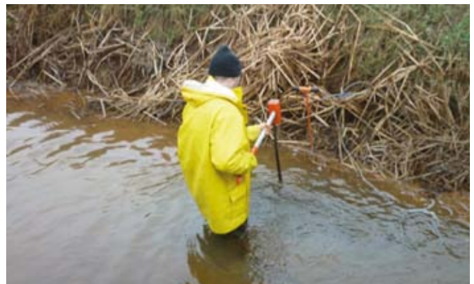
Figure 12. Installation of sensors in the riverbed to measure temperatures and heads to help determine fluxes across the groundwater-surface water interface.
