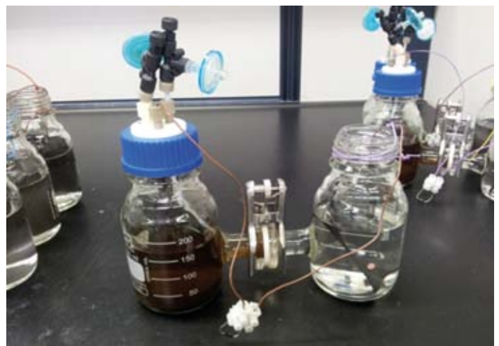
Figure 4. New microbial fuel cell reactor design
