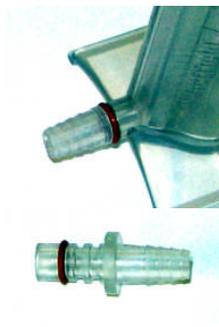
The **Sheffield LFC** flow-through cell comprises of a number of connected individual cells. Connections between cells are made water tight with o-rings.
