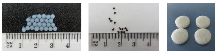
Figure 1. From the left, empty swollen beads, RSP-loaded dried beads and Thp-loaded beads compressed to tablets
