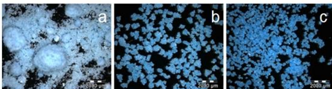
Three different lactose particle systems with a) fine, b) middle and c) big particle sizes treated with a blue coloured molten binder.
