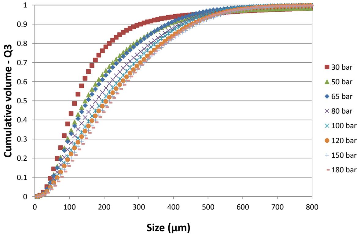
Figure 3. Cumulative size distributions of fragments of ribbon produced with powder at  $a_w=0.422$  after ball milling.
