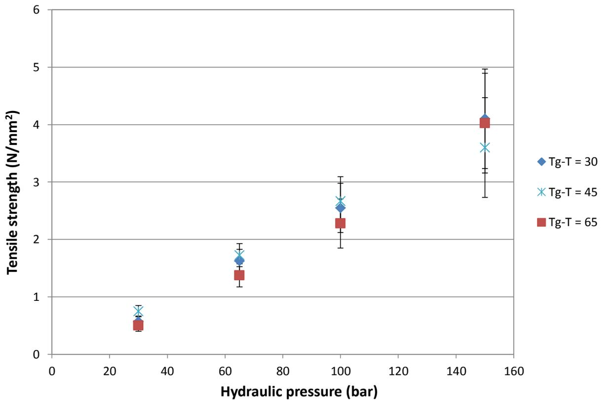
Figure 7. A plot of ribbon tensile strength against hydraulic pressure for each of the Tg-T values.
