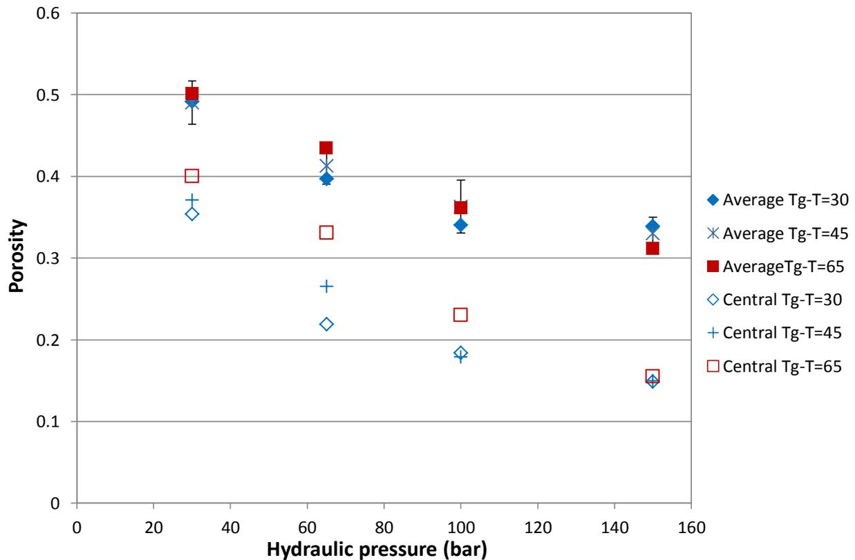
Figure 9. A plot of porosity against hydraulic pressure for each of the Tg-T values.
