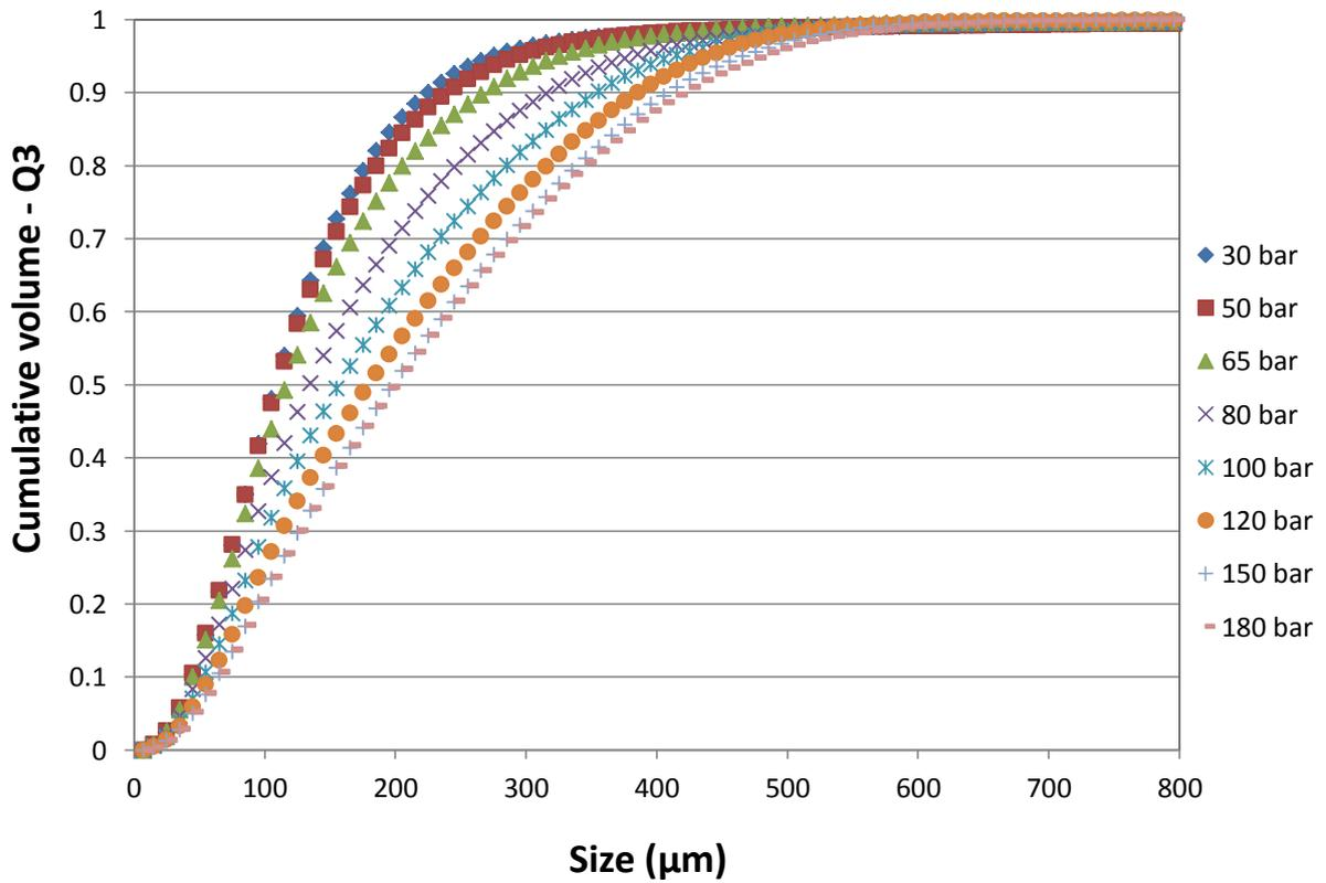
Figure 2. Cumulative size distributions of fragments of ribbon produced with powder at  $a_w=0.322$  after ball milling.
