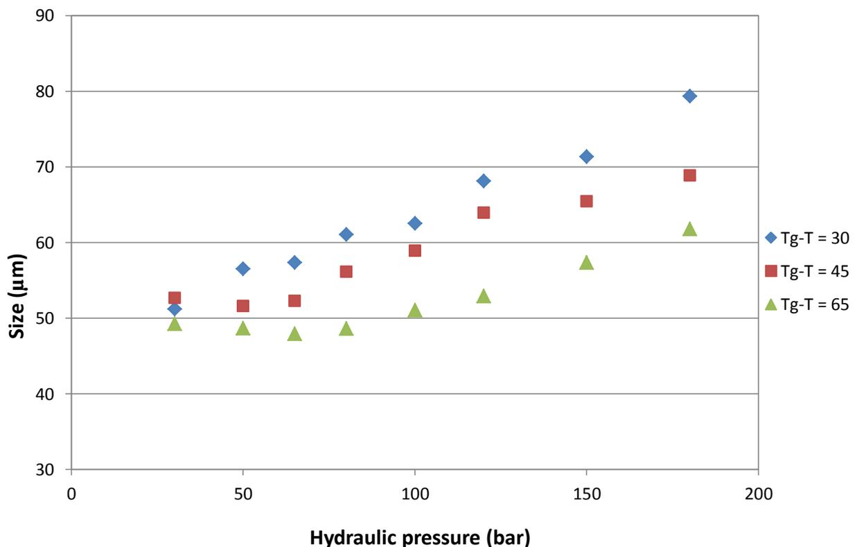
Figure 4. A plot of  $d_{10}$  against hydraulic pressure for each of the  $T_g-T$  values.
