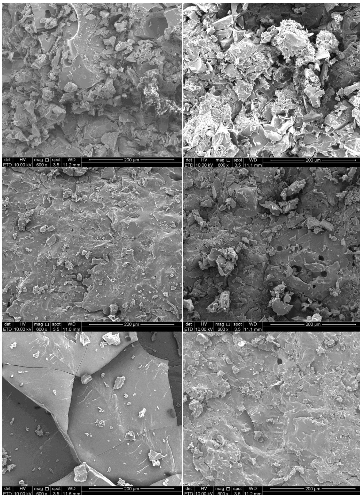
Figure 13. SEM images at 600x magnification showing the difference in structure between the ribbon produced at 30, 80 and 180 bar pressure (top, middle and bottom respectively) as well as the difference between powder at Tg-T=30 and Tg-T=65 (left and right respectively).
