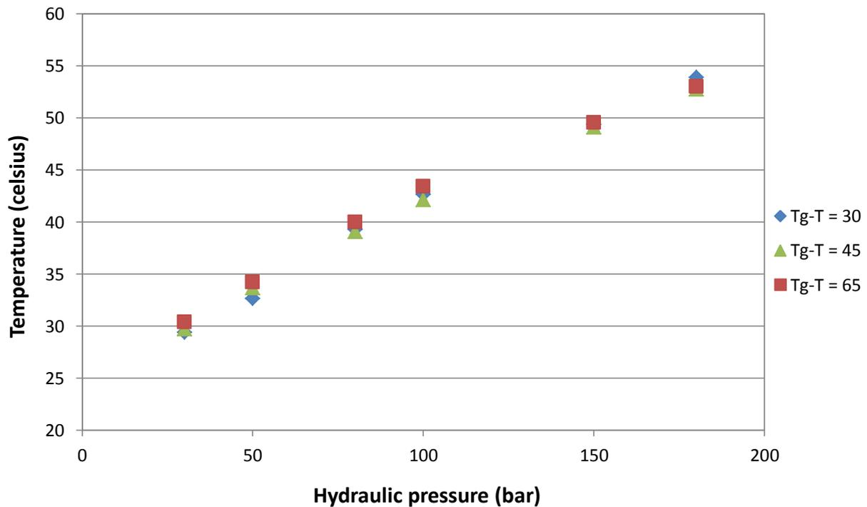
Figure 11. Ribbon temperature on exit of roller compaction using powders equilibrated to different water activities at 25°C.
