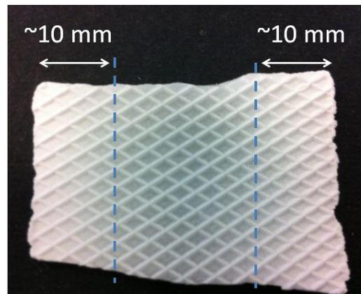
Figure 8. An image showing the method used for sectioning the ribbons.
