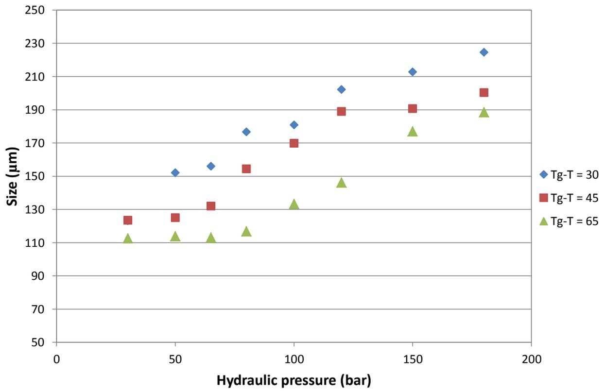
Figure 5. A plot of  $d_{50}$  against hydraulic pressure for each of the Tg-T values.
