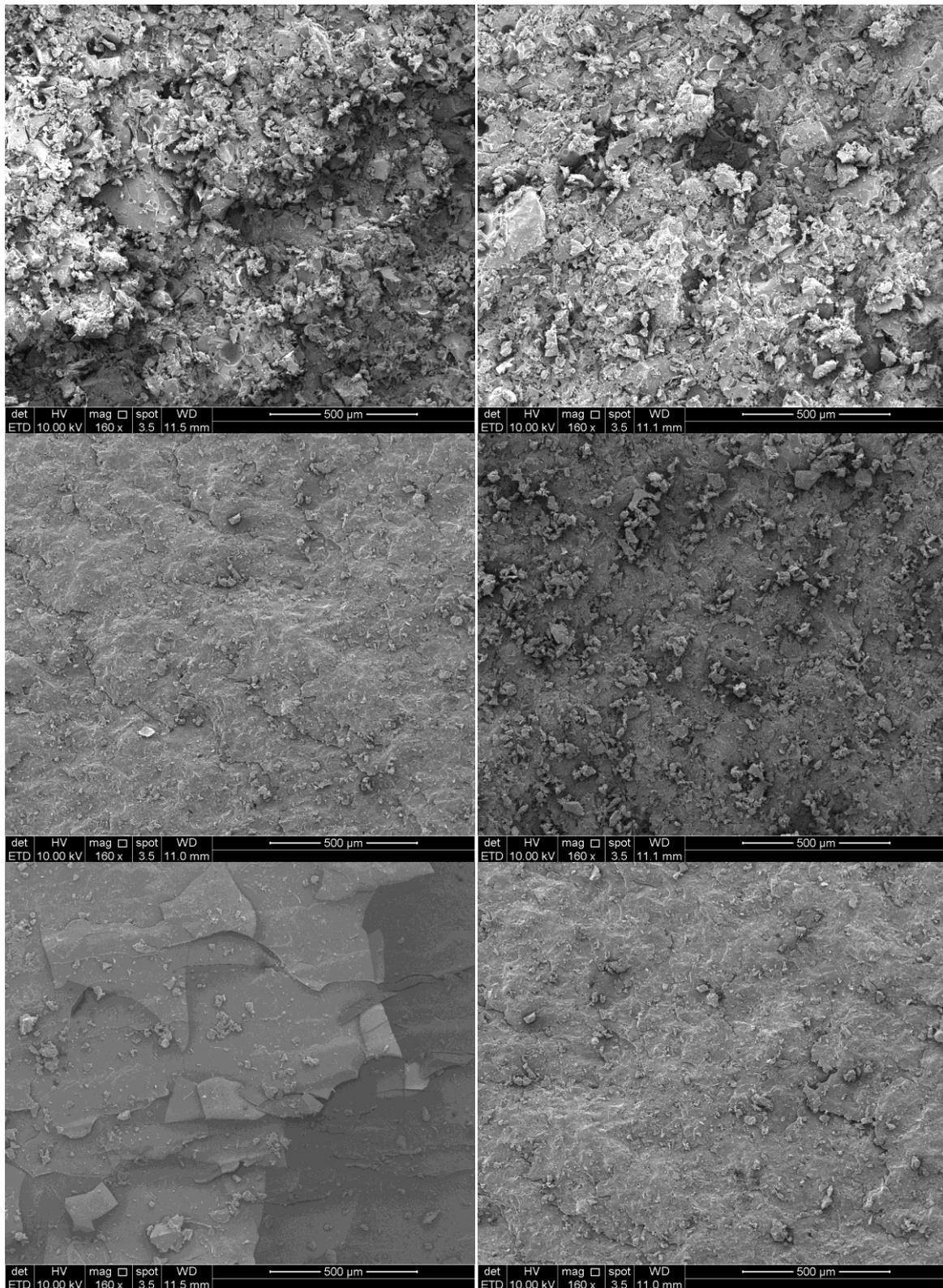
Figure 12. SEM images at 160x magnification showing the difference in structure between the ribbon produced at 30, 80 and 180 bar pressure (top, middle and bottom respectively) as well as the difference between powder at Tg-T=30 and Tg-T=65 (left and right respectively).
