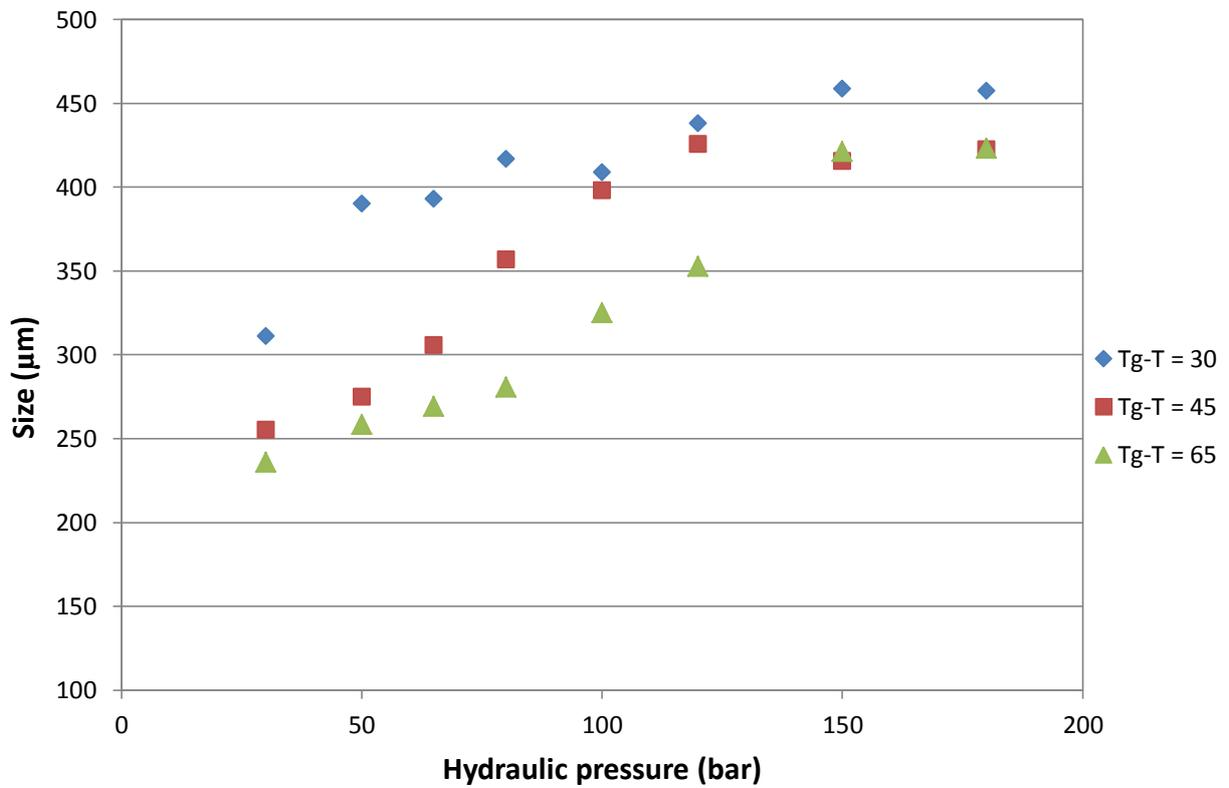
Figure 6. A plot of  $d_{90}$  against hydraulic pressure for each of the Tg-T values.
