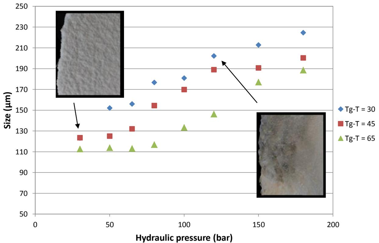
Figure 14. Optical images added to Figure 5 showing the difference in appearance of ribbon produced with powder at  $T_g-T=30$  for different hydraulic pressures (Left: 30 bar, Right: 120bar).
