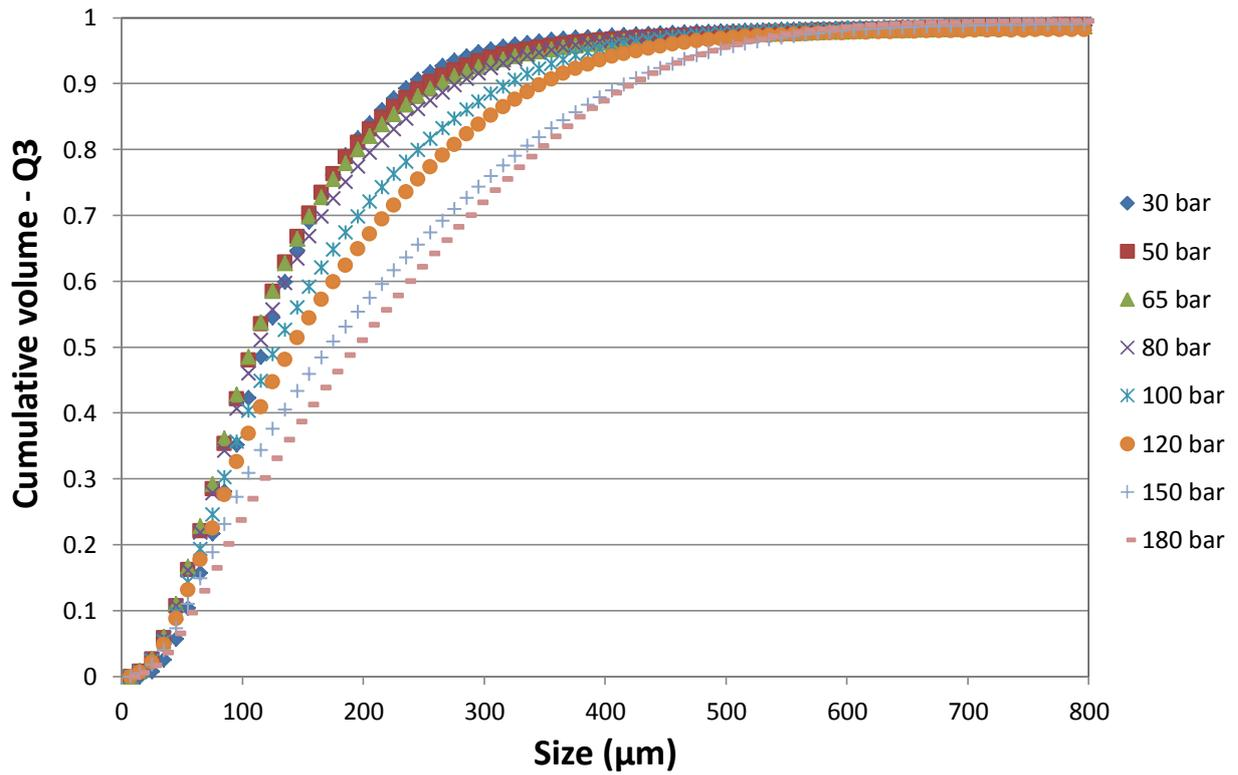
Figure 1. Cumulative size distributions of fragments of ribbon produced with powder at  $a_w=0.15$  after ball milling.
