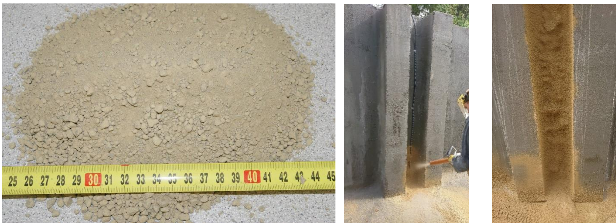
Figure 1: Granulated bentonite B75 REC MIX I in the laboratory (left) and pictures of the spray testing of B75 REC MIX for a sealing layer between concrete walls and soil dam at an experimental model.
